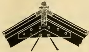
No. 2. The ridge, showing the wrought iron joining plate with the ridge rod cross tie support bolted to it.
