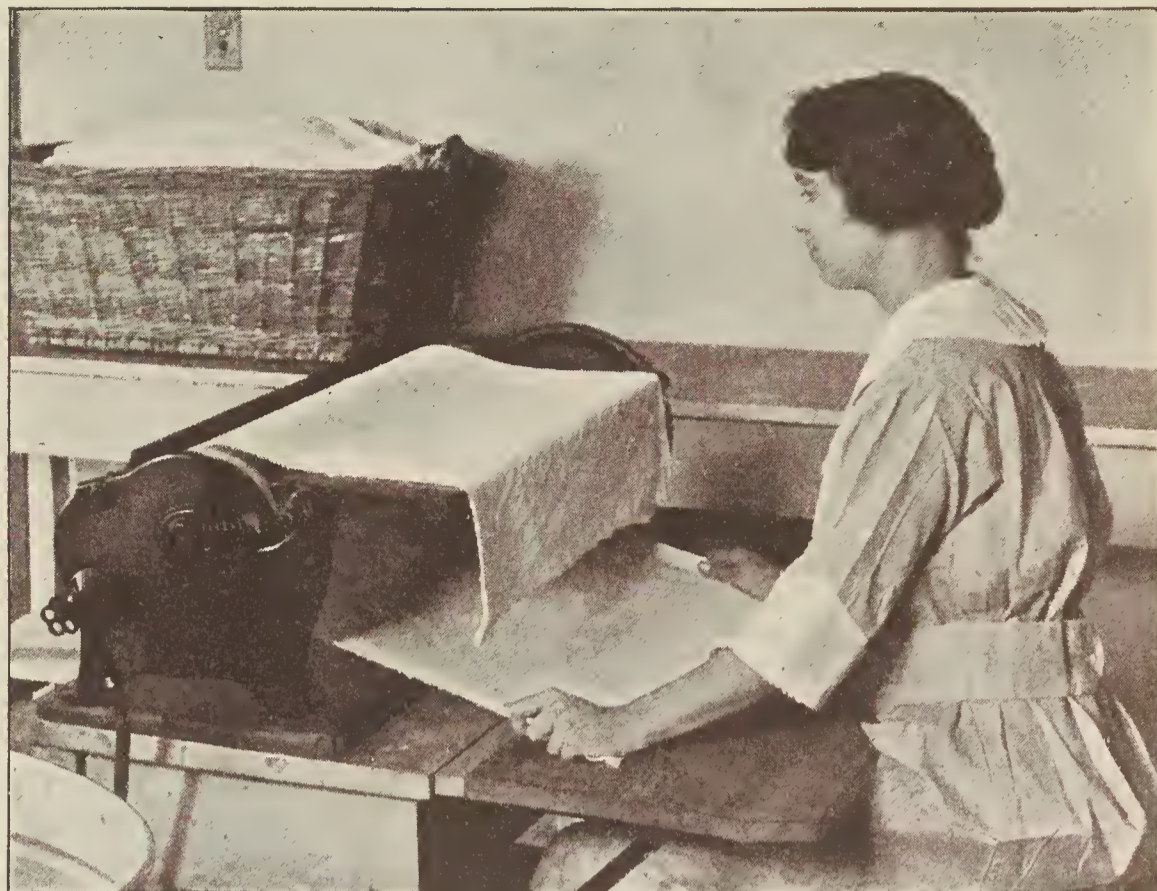
This mangle irons flat pieces between a heated steel and a padded cloth-covered cylinder. Mangles are turned by hand or by electricity and heated by gas or electricity
