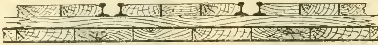
Fig. 12. Guard rails, used to make the rail heads even with the surface of the floor.
