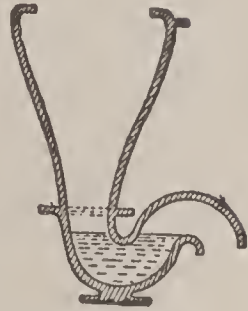
Figure 38. The hopper closet.
