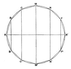
Then, if the polygon and great circle revolve together about the diameter AA', the angular points of the polygon, except A, A', will describe circles on the surface of the sphere at right angles to the diameter AA'. Also the sides of the polygon will describe portions of conical surfaces, e.g. BC will describe a surface forming part of a cone whose base is a circle about CC' as diameter and whose apex is the point in which CB, C'B' produced meet each other and the diameter AA'.
