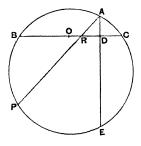
due to Archimedes, whatever may be said of the composition of the whole book. This proposition proves that, if in the first figure APR is so drawn that PR is equal to the radius OP, then the arc AB is three times the arc PC. In other words, if an arc AB of a circle be taken subtending any angle at the centre O, an arc equal to one-third of the given arc can be found, i.e. the given angle can be trisected, if only APR can be drawn through A in such a manner
