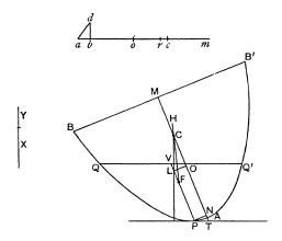
Let X + Y be a straight line such that (spec. gr. of solid) : (spec. gr. of fluid) =  $(X + Y)^2 : am^2 \dots (\alpha)$ , and suppose X = 2Y.
