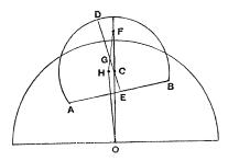
The centre of gravity of the portion of the segment outside the fluid, as F, lies on OC produced, its axis passing through C.
