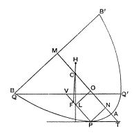
Make PF equal to 2FV, so that F is the centre of gravity of the immersed portion.
