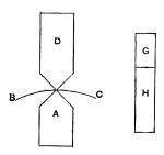
Therefore the weight of the fluid displaced is (G+H), and hence the volume of the fluid displaced is the volume of the solid A. There will accordingly be rest with A immersed and D projecting.
