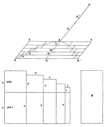
Then we can draw a cylinder or a frustum of a cylinder EBB'F passing through the circle or ellipse about BB' and having AD for its axis; also we can describe a cone or a segment of a cone through the circle or ellipse and having A for its vertex.
