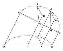
In the plane containing DE, OR describe a circle on DE as diameter. Through this circle (which must pass through R) draw a cylinder with axis OC.
