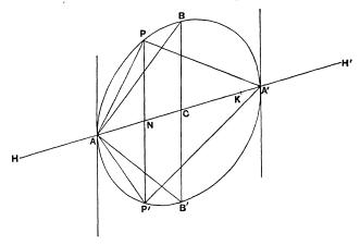
Draw the tangents to the ellipse which are parallel to PP'; let them touch the ellipse at A, A', and through the tangents draw planes parallel to the base of the segments. These planes will touch the spheroid at A, A', the line AA' will pass through the centre C and bisect PP' in N, while AN, A'N will be the axes of the segments.
