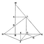
form an angle, and we now draw from the given point F a straight line FGK, meeting CG, CK in G, K respectively, such that the intercept GK is equal to AD or FC. (This is the  $\nu\epsilon\nu\sigma\iota$ s to which the problem is reduced, and it can be solved by means of a conchoid with F as pole.)
