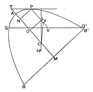
III. If the angle MTP is equal to the angle dab, the solid will rest in that position, because L and F will coincide, and all the forces will act along the one line CL.
