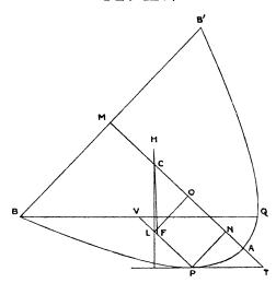
Thus F again lies between P and L, and, as before, the paraboloid will turn in the direction of diminishing the angle PTN, i.e. so that the base will be more submerged.
