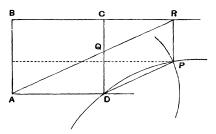
Therefore, to effect the construction, we have only to draw this rectangular hyperbola and the circle with centre D and radius equal to k. The intersection of the two curves gives the point P, and R is determined by drawing PR parallel to DC. Thus AQR is found.
