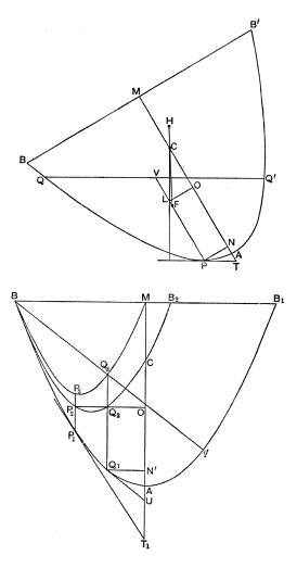
plane of the surface of the fluid in QQ'. Let PT be the tangent parallel to QQ', PV the diameter bisecting QQ', PN the ordinate at P.
