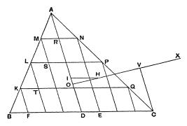
Divide both BD and DC into lengths each equal to DE, and through the points of division draw lines each parallel to DA meeting BA and AC in points as K, L, M and N, P, Q respectively.
