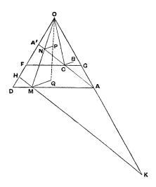
Lastly, draw MQ perpendicular to the plane of the paper (and therefore perpendicular to both HK and AD) meeting the ellipse or circle about AD (and therefore the surface of the cone) in Q.
