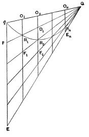
$R_n$  respectively. Through  $R_1, R_2, \dots R_n$  draw diameters of the parabola meeting qQ in  $O_1, O_2, \dots O_n$  respectively.
