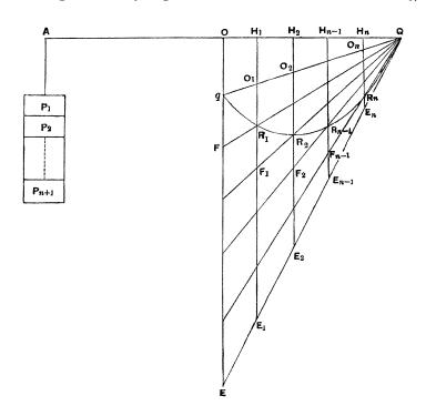
Suppose AO made equal to OQ, and conceive QOA as a lever placed horizontally and supported at O. Suppose the triangle EqQ suspended from OQ in the position drawn, and suppose that the trapezium  $EO_1$  in the position drawn is balanced by an area  $P_1$  suspended from A, the trapezium  $E_1O_2$  in the position drawn is balanced by the area  $P_2$  suspended
