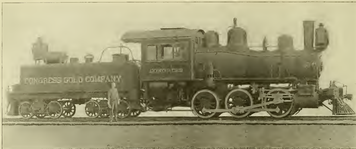
Switching Engine Burning Crude Petroleum.—Built by Brooks Locomotive Works
