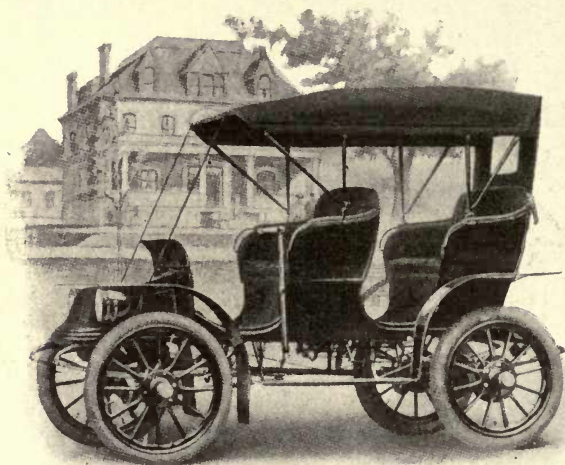
Fig. 159. Baker Electric Surrey, with Cape Top. Can be quickly converted into an inclosed vehicle in stormy weather. Baker Motor Vehicle Company, Cleveland, Ohio.
