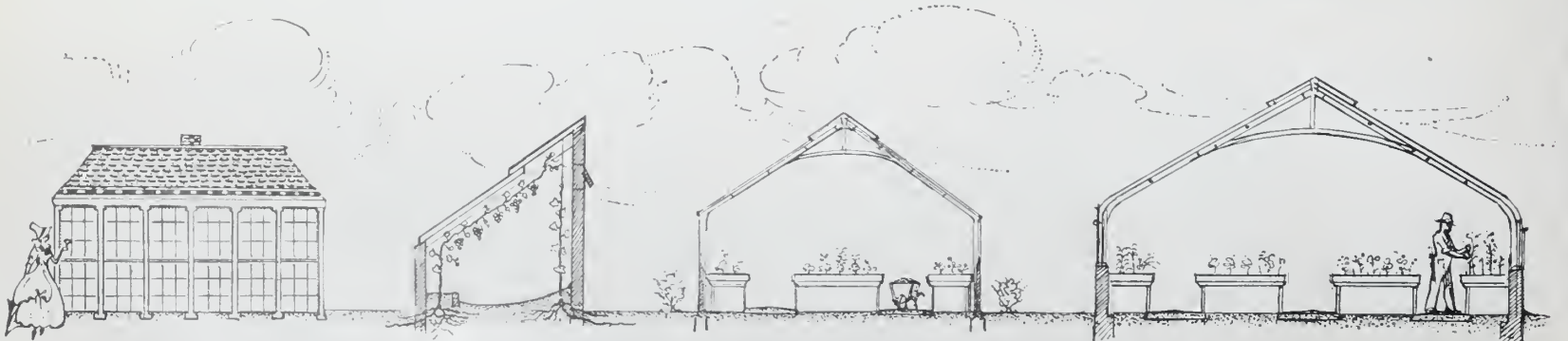
Greenhouse progress: The glasshouse of our ancestors; a lean-to grapery; a modern, all-steel 18 ft. house; an improved, curved-cave 25 ft. structure
