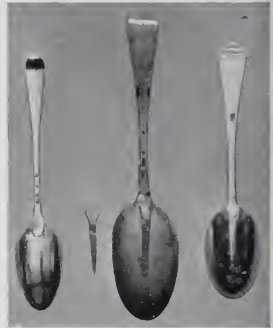
Left, dropped back spoon; center, rattail and spoon to be soldered together; right, finished spoon
