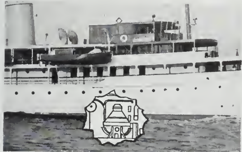
DIAGRAMMATIC VIEW OF GYROSCOPE One of the largest ever installed in a yacht, the stabilizer is both efficient and out of sight.
