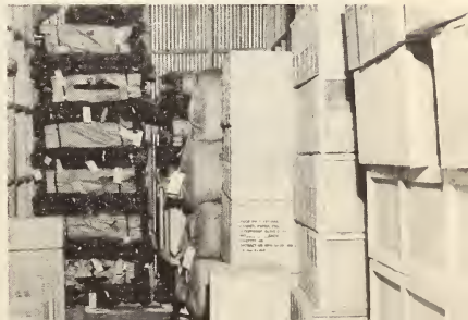
Stacks of folded cots plus over 600 crates and boxes comprise a 62000 Series PDH in storage. About 7500 cubic feet of storage space is required.
