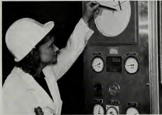
6 Canned chili and soups are often made in high-tech processing operations. Equipment like this retort or pressure cooker is used to cook products to high temperatures, destroying any foodborne pathogens that may be present. Botulism is a major concern because botulinum bacteria form spores that only high temperatures kill. In addition to making sure products are cooked at proper temperatures, food technologists check a number of other safety factors....
