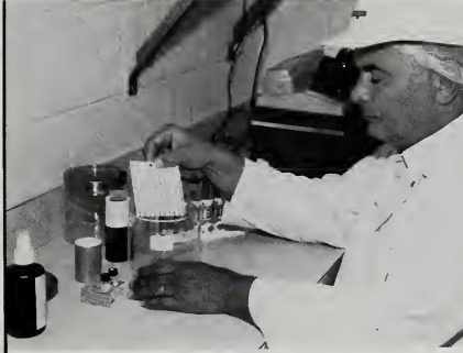
4 Inspection includes checking for drug and chemical residues in animal tissues. Residues can result from the improper use of pesticides and animal drugs as well as industrial and environmental accidents. In some cases, quick tests are used in the plant to check for residues. This veterinarian is using the Sulfa-On-Site quick test to check the animal's urine for a sulfa drug. It can detect the drug within 45 minutes.
