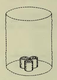
Fill the three small cans with insulating material. If glass fiber is used, wear gloves and long sleeves, as the small particles of glass are apt to prick the skin. Place the three cans about 1 inch apart in the center of the bottom of the outside container. the bottom of the container with the insulation up to the top of the small cans.
