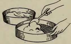
When the concrete has set so that water does not coze out of it, scoop out enough concrete to expose the wire loop. Let stand for 2 or 3 days before removing the cardboard form. Before using the stone it must be tempered by placing in boiling water for 15 minutes. Let it dry again for approximately 2 days.
