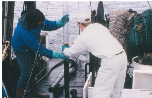
Taking a sediment core in Narragansett Bay. Winching the corer up (Top). Cutting the excess plastic off above the top of the sediment (Bottom). Photo courtesy of EPA Atlantic Ecology Division.
