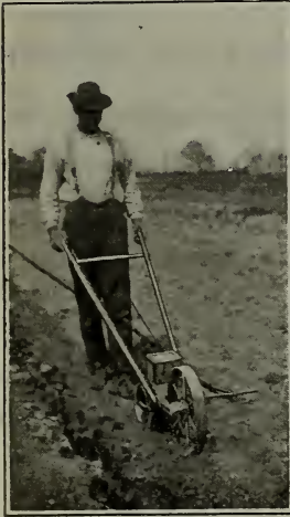
Planet Jr. No. 25. Hill and Drill Seeder at work planting and marking next row.
