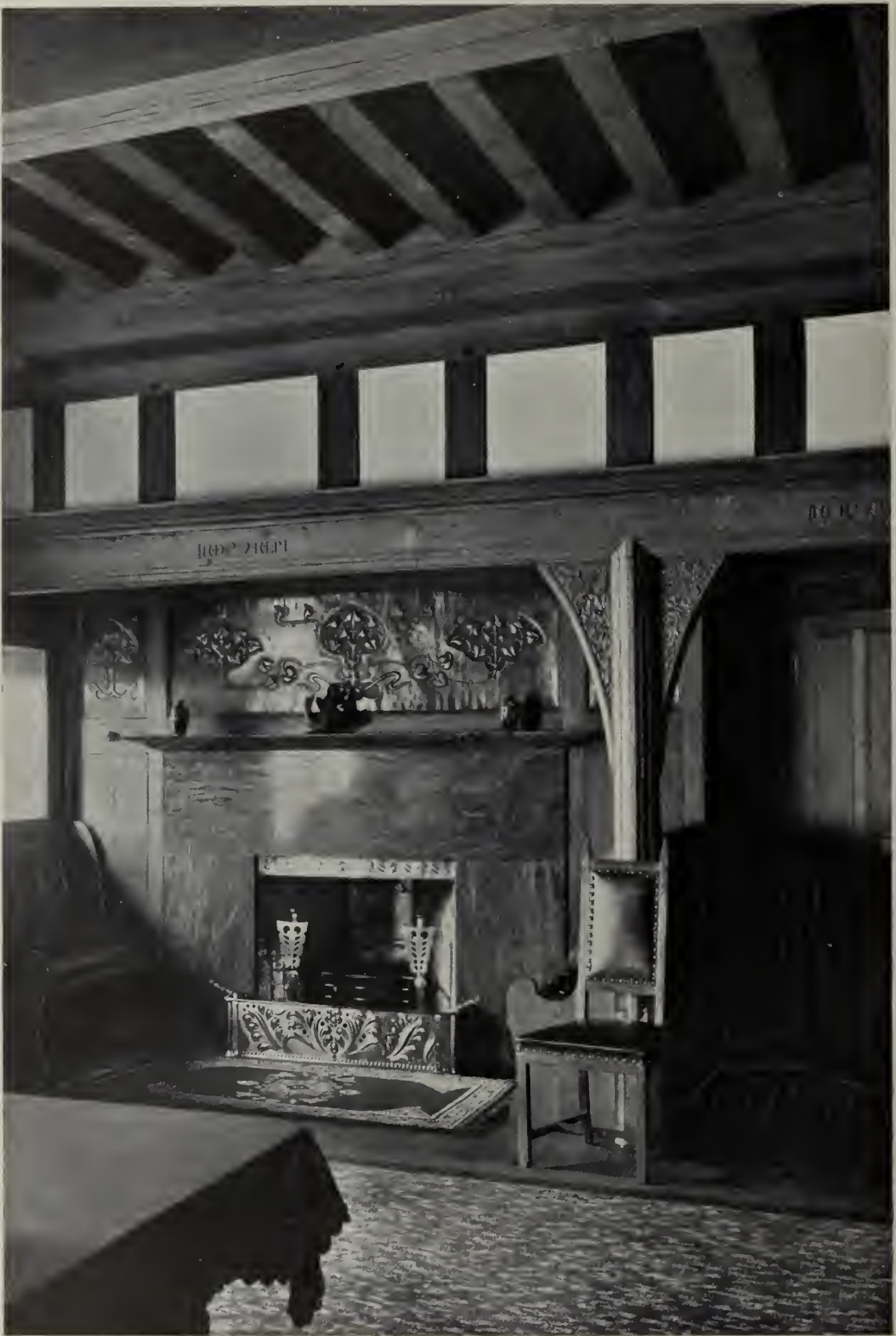
THE DINING-ROOM FIREPLACE AT BRAHAN, PERTH. THE INGLENOOK AND THE CEILING ARE OF SOLID OAK BEAMS AND THE PANELS OVER THE FIREPLACE ARE IN COPPER BY MR. EDGAR SIMPSON. SLABS OF IRISH GREEN MARBLE SURROUND THE FIREPLACE. THE GRATE IS OF BRIGHT STEEL
