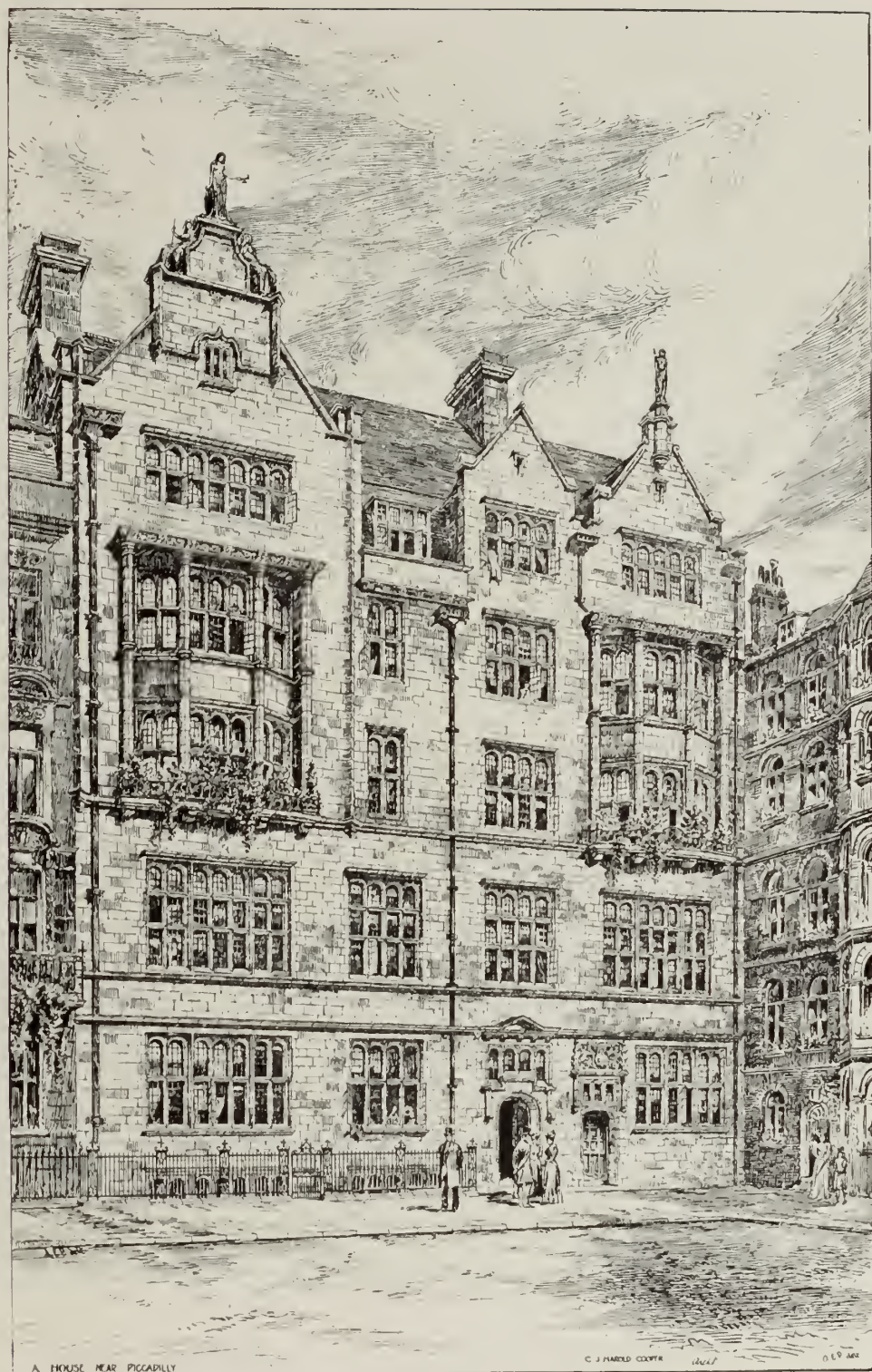
ORIGINAL DESIGN FOR A HOUSE NEAR PICCADILLY, BUILT OF PORTLAND STONE. THE RAIN-WATER HEADS ARE OF BEATEN LEAD, BY T. STIRLING LEE
