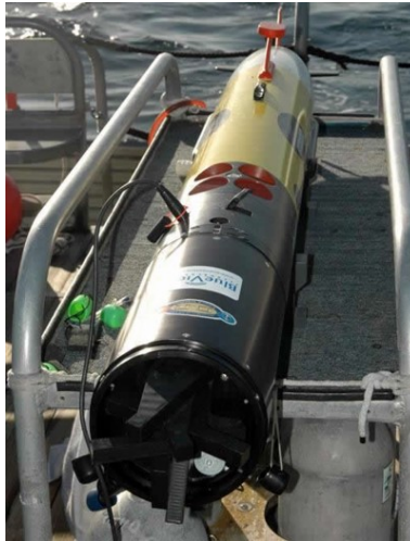
Figure 1.3. The Remus 100 UUV platform.
