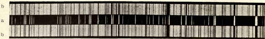
FIG. 1—Coincidence of bright lines (a) from iron vapor with dark lines (b) in the Sun's spectrum, violet region, \lambda 4200 .
