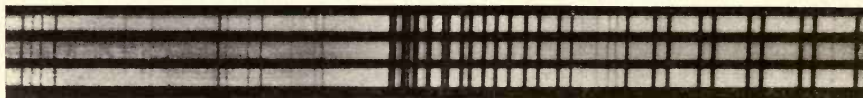
FIG. 3—Lines of B group due to oxygen in the Earth's atmosphere undisplaced by Sun's rotation, red region, \lambda 6867 .
