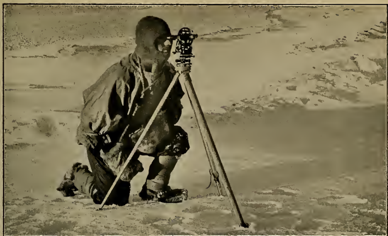
LIEUT. EVANS SURVEYING WITH THE THEODOLITE USED BY CAPT. SCOTT TO LOCATE THE SOUTH POLE.
