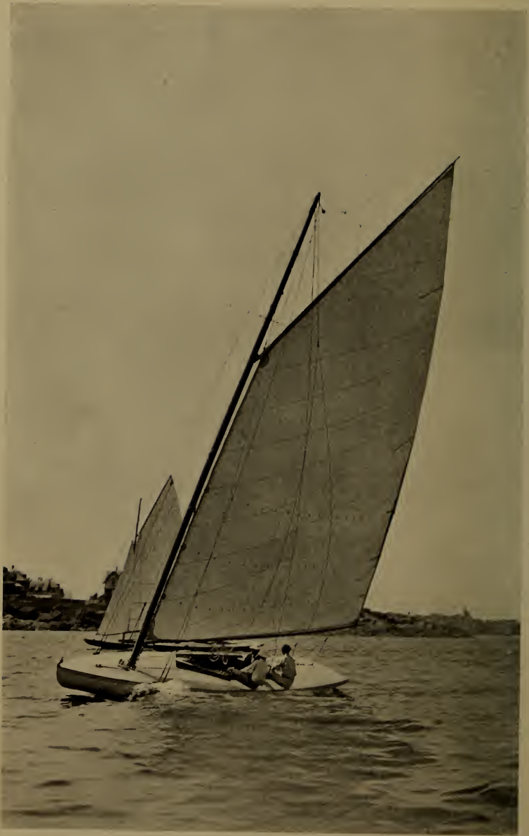
Sonder Class boat with cat rig. A fast rig to windward in smooth water but of no use in other conditions. 550 square feet of sail in the mainsail
