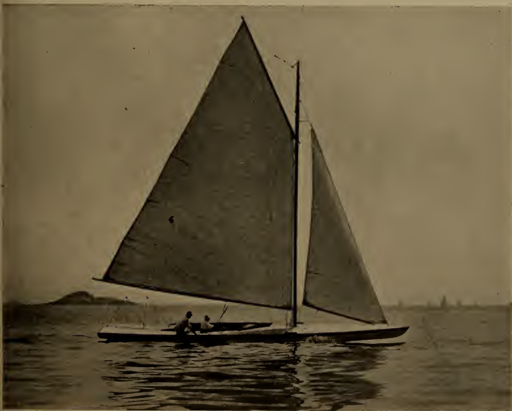
A flat formed, low ended Sonder Class boat, showing lifting tendency of bow wave even in very light weather
