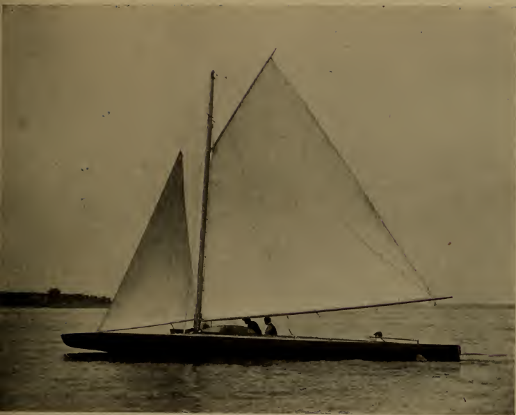
Windward side, showing long straight sailing lines and port rudder Weather bilge-board hoisted
