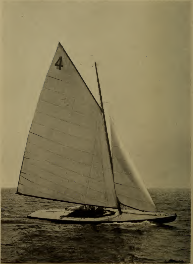
On a close reach at good speed. Easy formed scow Sonder boat. First choice for the American team of 1906. A very fast boat in light weather. Note especially smooth wake
