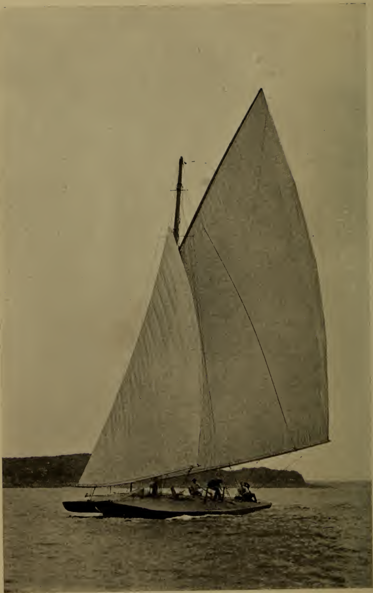
Three hulled boat built on wire trusses on 21-foot water line with 2000 square feet of sail. She was impossible to handle in anything other than very light weather, having no ballast
