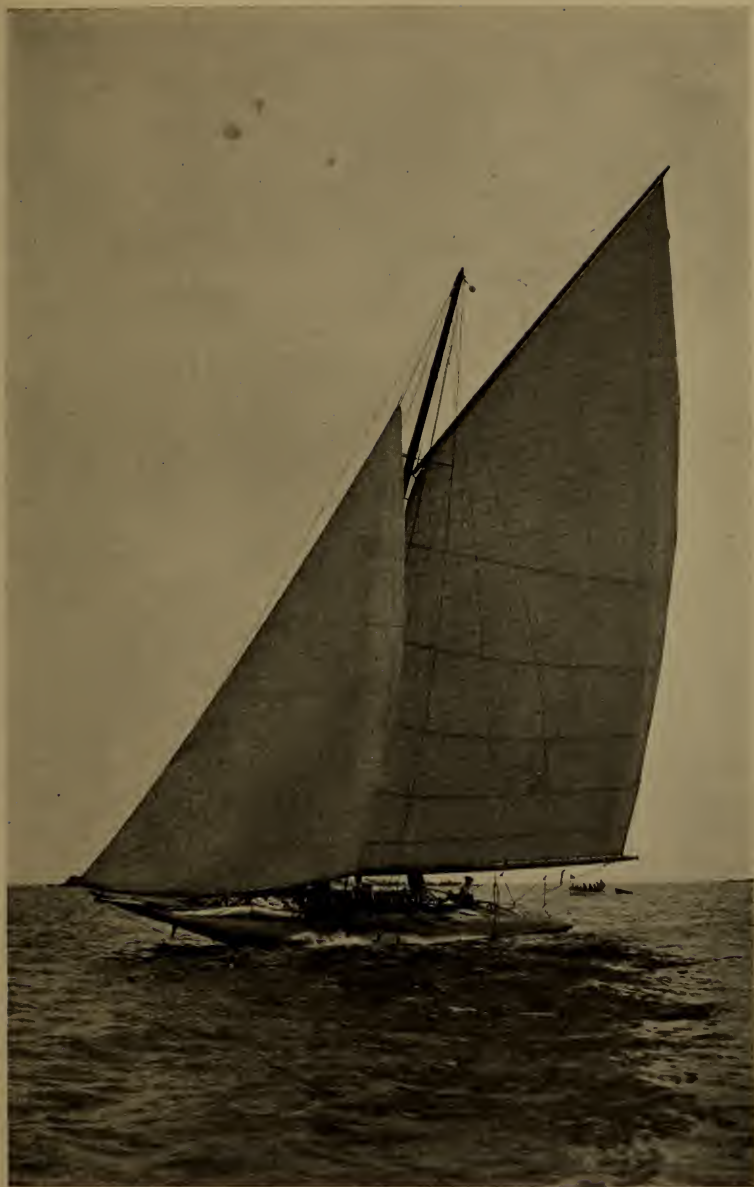
21-foot water line unrestricted racing scow, 50 feet over all, 1900 feet of sail in mainsail and jib. Built on steel truss. About the limit that this type can go and still hold together
