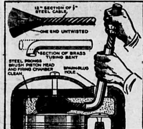
A Carbon Remover Which Has a Very Direct and Positive Action Is Made From Stranded Steel Cable.
