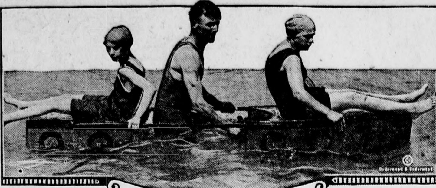
David Swarhout and James Smith of Evanston, Ill., have built a "bicycle pontoon" which is here seen carrying two passengers. It consists of two air-tight tin tanks and a bicycle frame. The pedals turn a sprocket wheel and chain, thus revolving the screw.
