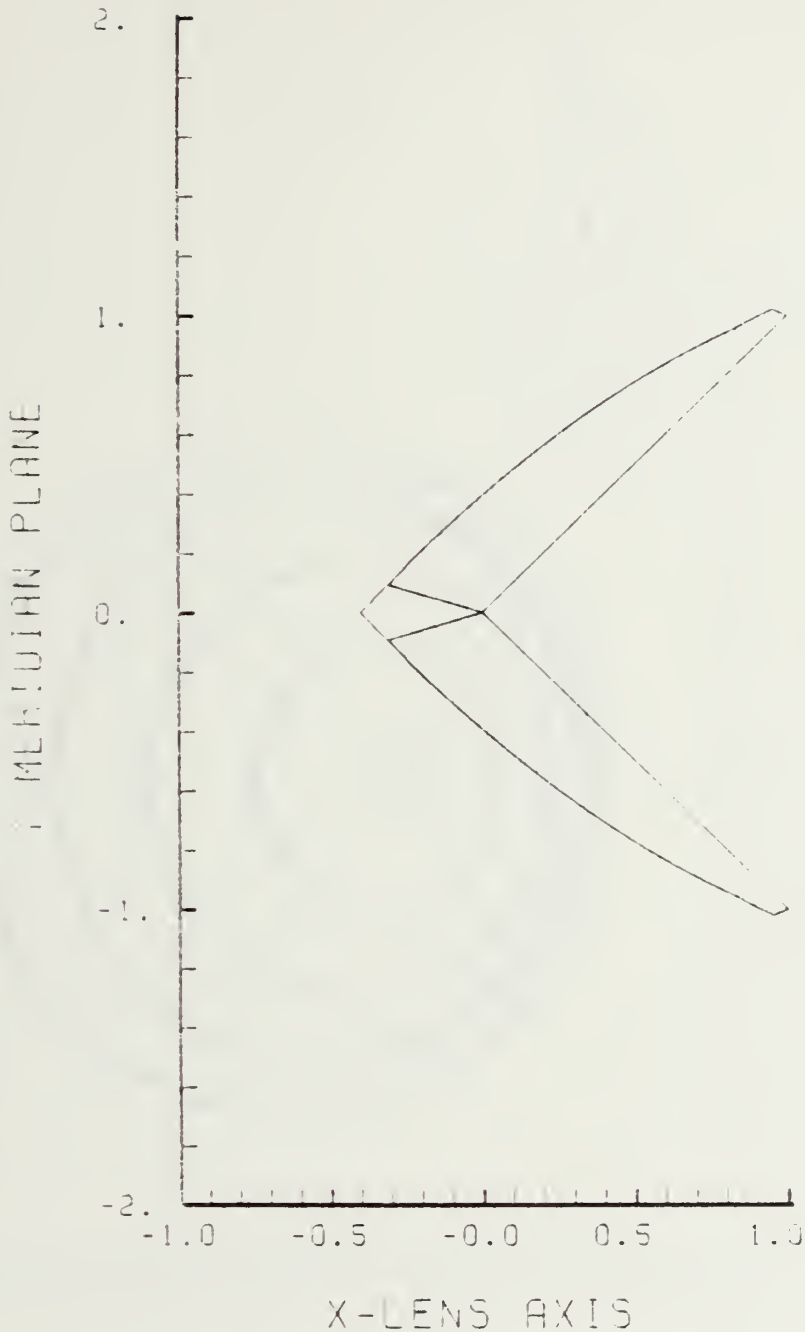
Figure E-33. GRIN Lens Shape at -10%, OB = 0.30, a = 2.25
