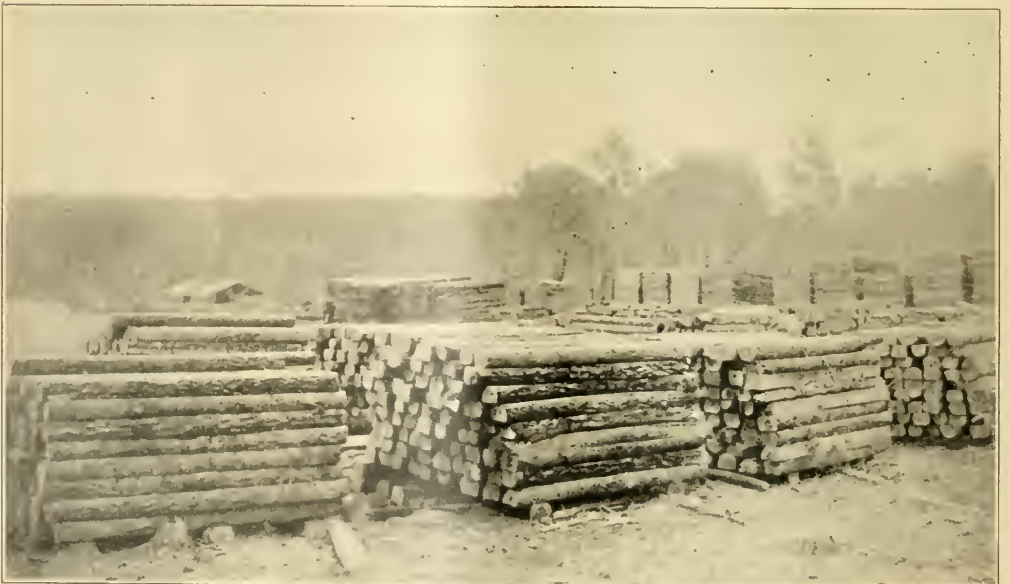
MARITIME PINE RAILWAY TIES PILED READY FOR SHIPMENT ; ALSO LUMBER PRODUCED AT AMERICAN SAWMILL IN MARITIME PINE FOREST IN SOUTHWESTERN FRANCE
