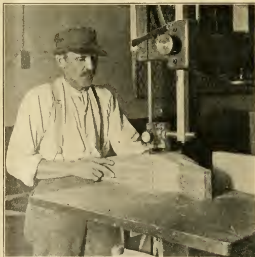
IN THE MANUFACTURE OF LAMINATED BOWLING PINS THE MATERIAL OF THE PROPER SIZE AND KIND IS FIRST SURFACED ON TWO SIDES AND THEN GLUED UP INTO A BLOCK AND SET ASIDE FOR A WEEK OR LONGER TO ENABLE THEM TO REACH A STATE OF EQUILIBRIUM.
