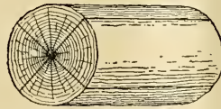
Shows manner of splitting timber into stave bolts where timber is of small diameter.
