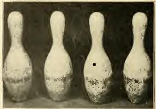
AFTER 250 GAMES THESE LAMINATED BOWLING PINS ARE STILL IN SERVICEABLE CONDITION, IN FACT THIS PARTICULAR SET IS, TO ALL INTENTS AND PURPOSES THE EQUAL OF SOLID PINS.
