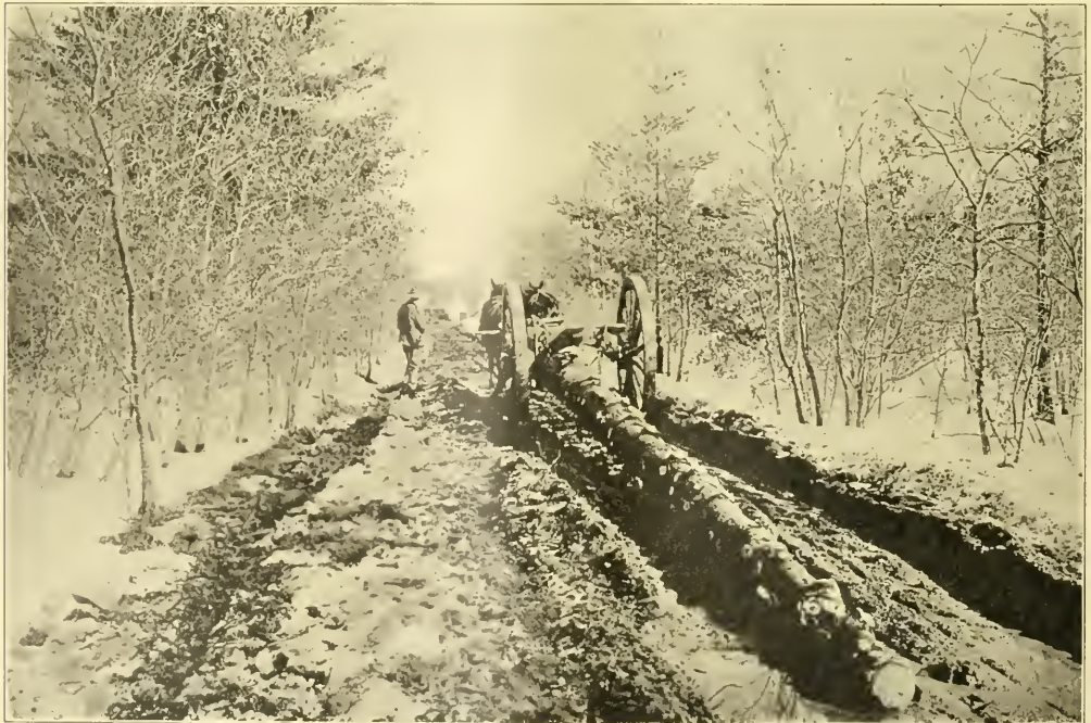
20th ENGINEERS IN FRANCE HAULING A SPRUCE TREE FULL LENGTH BY MEANS OF BIG WHEELS FROM WOODS TO MILL. OAK COPPICIE AT THE SIDES OF THE ROAD.
