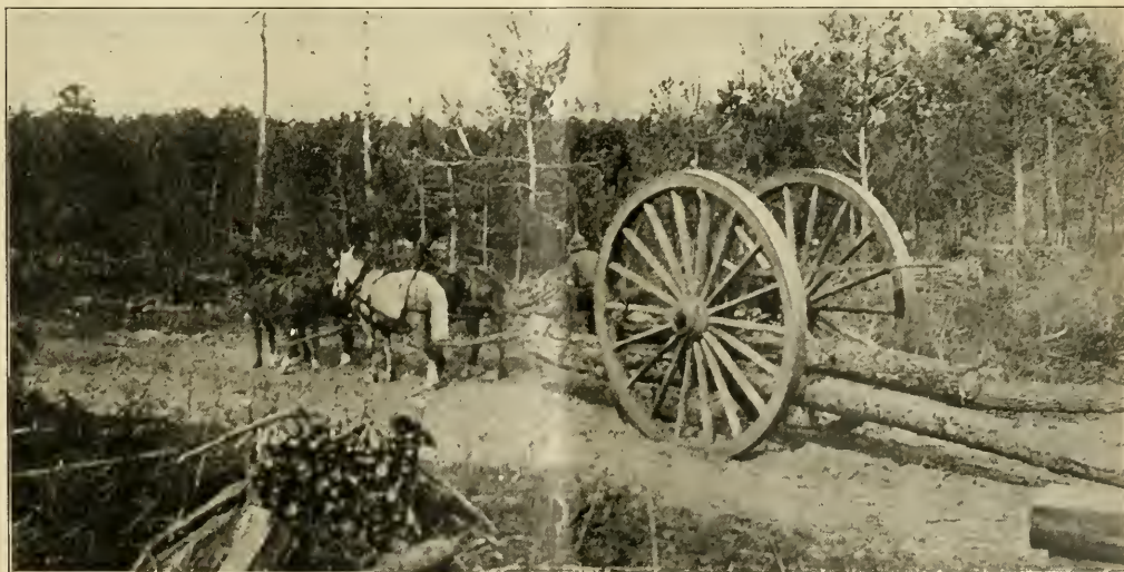
20th REGIMENT MEN TRANSPORTING LOGS, BY MEANS OF "BIG WHEELS," TO THE BANK OF THE COURANT RIVER, AUREILHAN OPERATION, NEAR PONTENX, LANDES, FRANCE
