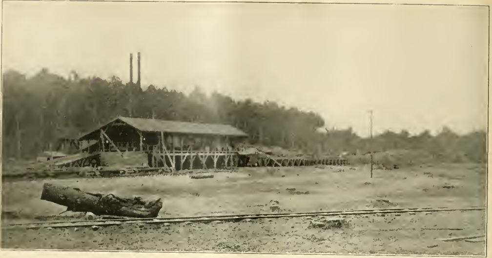
VIEW OF THE MILL YARD OF THE BOURICOS 20-M AMERICAN MILL NEAR PONTENX, LANDES. A LOG TRAIN HAS JUST BROUGHT THE LOGS OVER THE NARROW GAUGE RAILWAY SYSTEM FROM THE FOREST TO THE POINT WHERE THE LOGS WILL BE UNLOADED ON TO THE SKIDS IN THE FOREGROUND, OVER WHICH THE LOGS WILL BE ROLLED TO THE CARTS AT THE LEFT, UPON WHICH THEY WILL BE PULLED UP THE INCLINE INTO THE SAWMILL. THE GREAT HEAP OF SLABS AND EDGINGS AT THE RIGHT OF THE LOG TRAIN ARE DESTINED TO BE MADE INTO CHARCOAL FOR USE IN A NEARBY MUNITIONS PLANT.
