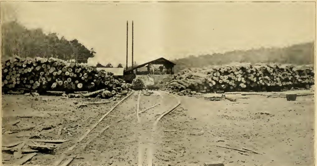
VIEW OF BOURICOS 20-M AMERICAN SAWMILL NEAR PONTENX, LANDES, SHOWING LOGS ON SKIDS READY TO BE TAKEN INTO THE SAWMILL
