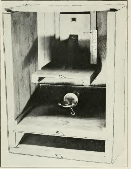
Fig. 20.—A form of the apparatus required for the preparation of Laue photographs. A and B are pinhole lead slits: the crystal holder (permits setting the section of the crystal at any desired orientation, D is a morable plate holder. Other and more complicated forms have been used; this cone is desired because of this simplicity.
