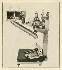
FIG. 12.—An X-ray spectrometer. G is a divided circle upon which the positions of the crystal and ionization chamber may be read: F is a microscope and scale for following the gold leaf of the electroscope (E); H is an earthed shield for the wire connecting the chamber and the electroscope.
