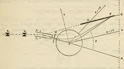
FIG. 1 .--- Theory of the mass-spectroscope.
