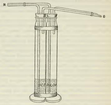
FIG. 2.--Apparatus for preparation of ammonium chloride sublimate.
