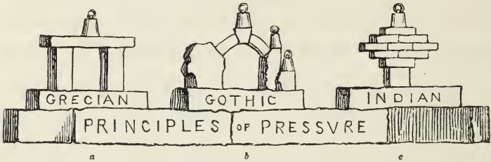
[Fig. 131. Sketch exhibiting the principles of pressure in Grecian, Gothic, and Indian architecture: a, Grecian b, Gothic; c, Indian.]
