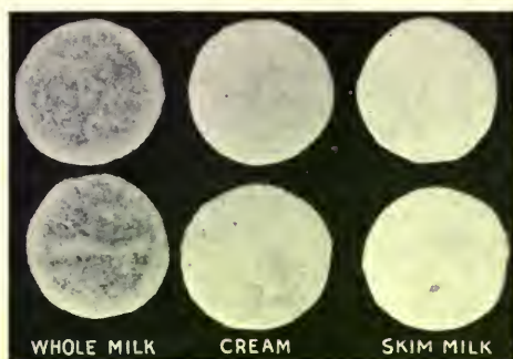
Fig. 78.—Sediment in milk before and after separating. The left column shows sediment from a pint sample of whole milk. The center shows that there is no sediment in newly separated cream from the same milk, and the right shows the test for the skimmed milk. This test was made at the factory. (Wisconsin Circular No. 41.)
