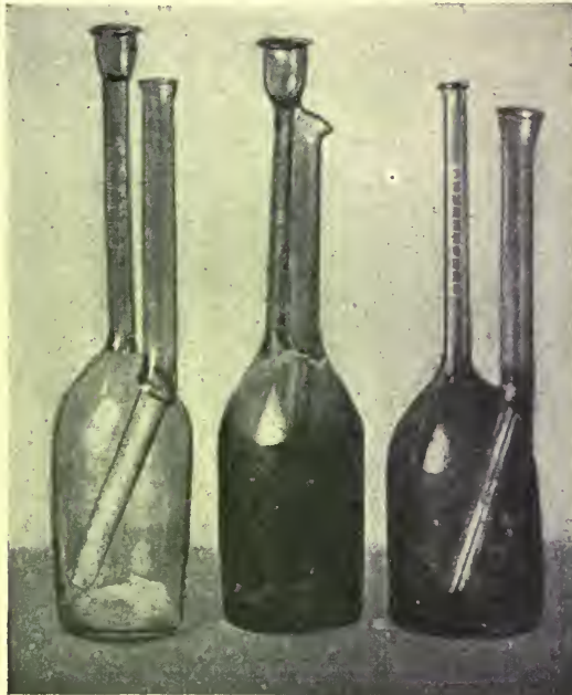
Fig. 64.—Test bottles used with skimmed milk and whey. Each division of the scale represents 0.05 per cent. on the neck of the bottle at the right. On the two bottles at the left each division represents 0.01 per cent. fat. (Circular of Information No. 27, July, 1911, Univ. of Wis. Agri. Exp. Sta.)
