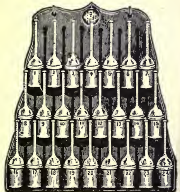
Fig. 62.—Rack for holding Babcock test bottles. (A. H. Barber Creamery Supply Co.)
