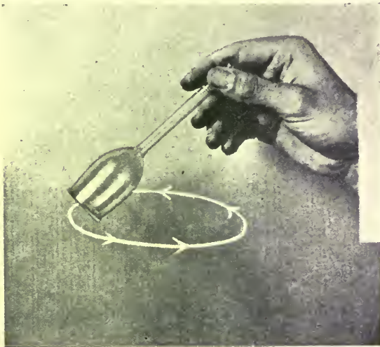
Fig. 43.—To mix the acid and milk shake the bottle until the contents are of a uniform brown color. (Circular of Information No. 27, July, 1916, Univ. of Wis. Agri. Exp. Sta.)
