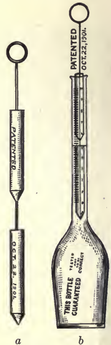
Fig. 49.— a , Milk-bottle tester; b , testing accuracy of milk bottle (Van Slyke).
