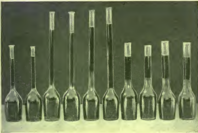
Fig. 46.—Types of cream and milk test bottles, showing fat columns, menisci, etc. (Bulletin No. 58, B. A. I.)
