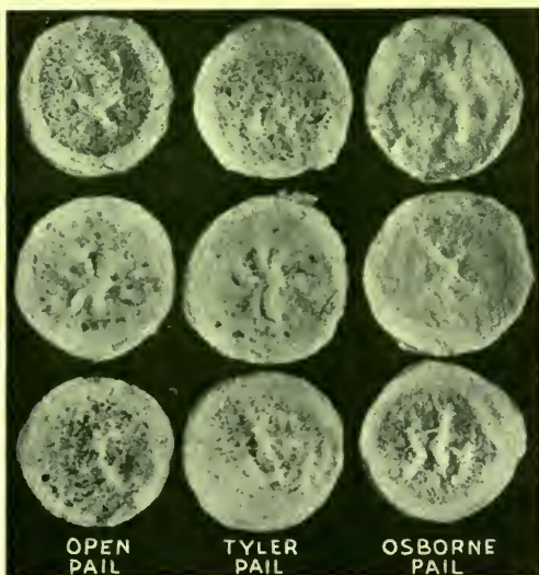
Fig. 79.—Open-top pails catch dirt. The larger the open top, the more dirt it catches. (Wisconsin Circular No. 41.)
