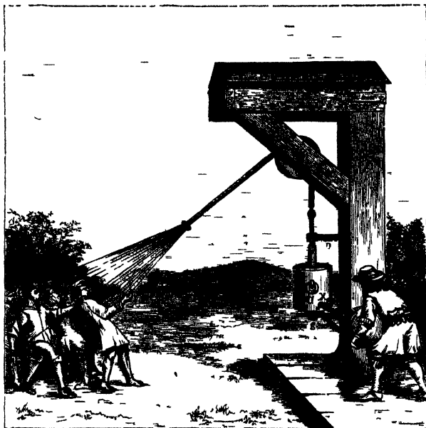
FIG 3 —GUERICKE'S CYLINDER AND PISTON MACHINE, 1654.
