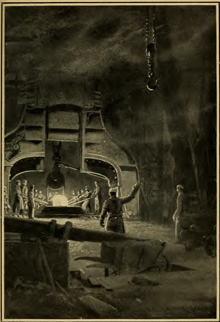
A steam hammer at work in Woolwich Arsenal, forging a steel ingot for the inner tube of a big gun. It delivers a blow equivalent to the momentum of a falling mass weighing 4000 tons. As speech is inaudible, the foreman gives hand signals to direct his men, who wear large canvas fingerless gloves to protect their hands from the intense heat.
