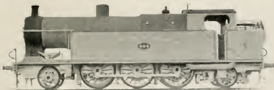
SIX-WHEELS-COUPLED SUBURBAN TANK ENGINE, L. AND Y. R.
