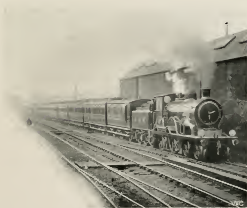
OIL-BURNING LOCOMOTIVE WITH TRAIN, G. E. R.
