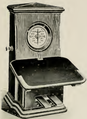
THE ELECTRIC TELEGRAPH INSTRUMENT NOW MOST EXTENSIVELY USED IN THE TRANSMISSION OF RAILWAY MESSAGES — VIZ., THE "SINGLE NEEDLE."
