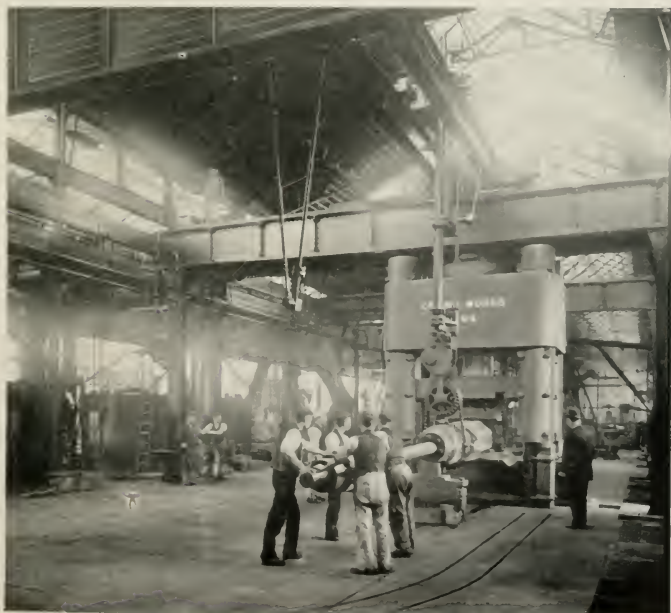
FORGING AN AXLE UNDER A 2,000-TON PRESS AT CREWE LOCOMOTIVE WORKS.
