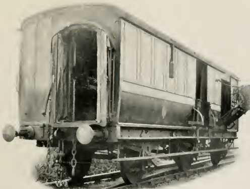
MAIL-VAN, SHOWING NET AND VESTIBULE CONNECTION, L. AND N. W. R. The net is used in connection with the apparatus shown below.
