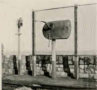
APPARATUS FOR SINGLE-LINE WORKING, G. W. R. Showing the position of the "staff," after it has been dropped from the train
