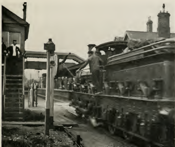
APPARATUS FOR SINGLE LINE WORKING. ENGINE-DRIVER PICKING UP "STAFF" AT SPEED, G. W. R.
