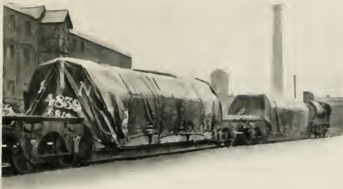
CONVEYANCE OF GLASGOW DISTRICT SUBWAY CABLE, 7 MILES LONG, BY L. AND N. W. R.
