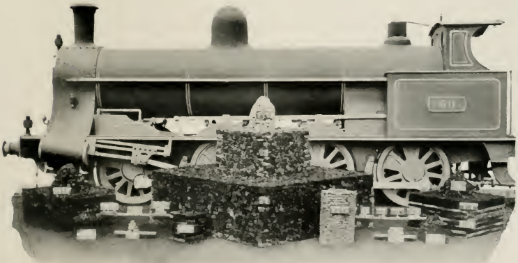
EIGHT-WHEELS-COUPLED MINERAL ENGINE, L. AND N. W. R.
