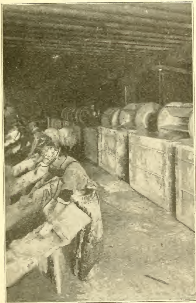
Beam house and pickling room, where the pelts are washed and the wool removed.
