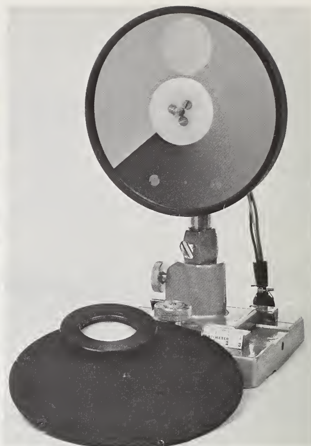
FIGURE 4. Close view of the circular, neutral wedge. The front plate which carries the fused silica lens was removed to show the fused silica disc with the evaporated metal layer.
