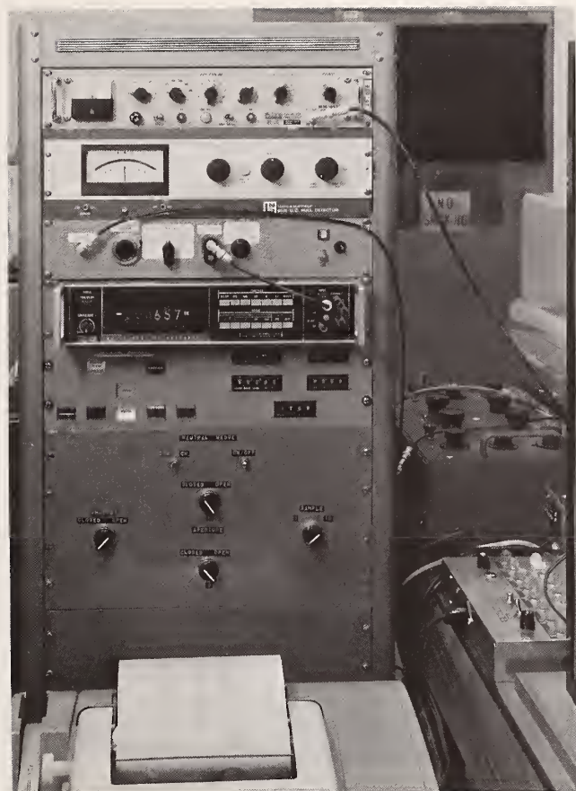
FIGURE 14. Console containing the power supply for the photomultiplier tube, the dc null detector, the current-to-voltage converter, the digital voltmeter, the command panel for computer operation, and the command panel for the pneumatic operation of the shutter, aperture system, and single sample carriage. The electric switches for operating the circular neutral wedge are also located on this panel.
