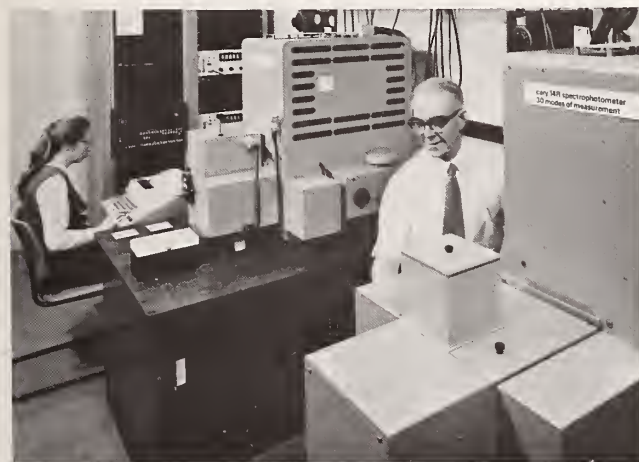
PLATE 5. View of the NPL on-line spectrophotometry data-system, showing the dedicated Micro 16P computer with 16K of core to which the two spectrophotometers shown in the foreground are interfaced in a time-sharing mode for independent operation and processing.
