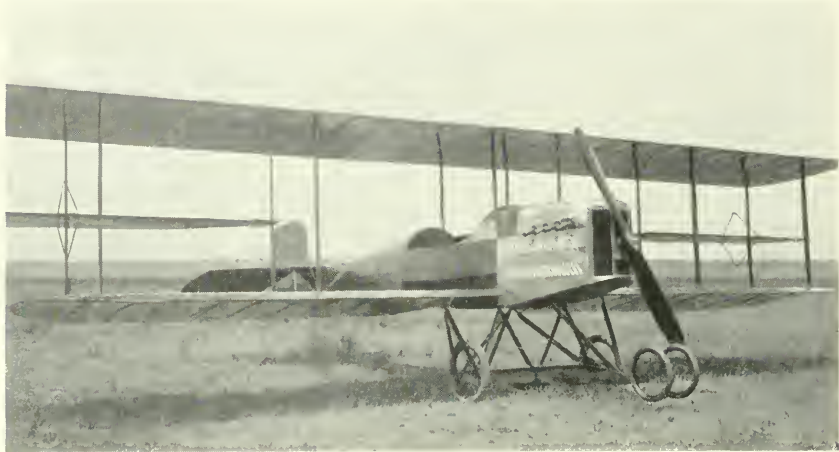
1. America's first highly successful tractor type, the Glenn Martin training plane of 1913. Note useless skids and nose wheels on the landing gear; also ailerons between the wings.
