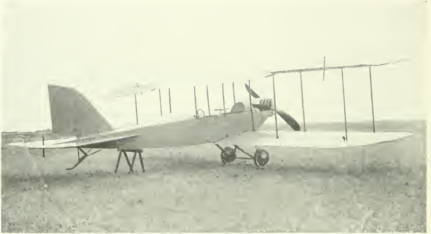
1. The first American simple two-wheel, no-forward-skid landing gear shown here was built by the author in San Diego in late 1913, and was later adopted for all Army aircraft.
