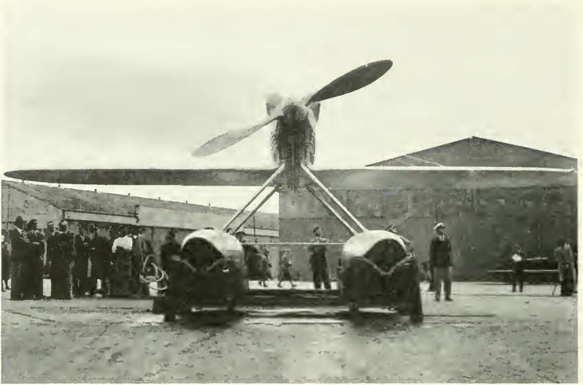
1. The world's-record supermarine seaplane (1929). Necessary propeller clearance and high center of gravity made this a heavy, awkward plane, with greatly added head resistance.
