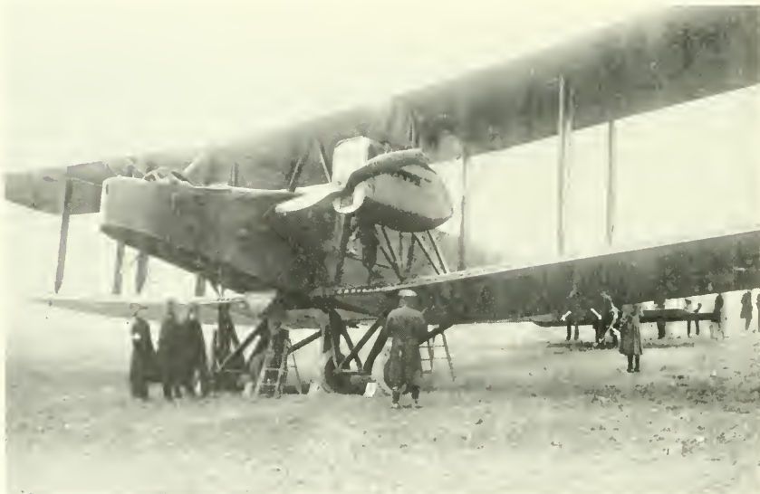
2. The Handley-Page of World War I. This widely used twin-engine plane typifies the configuration of engine between the wings at this early stage.
