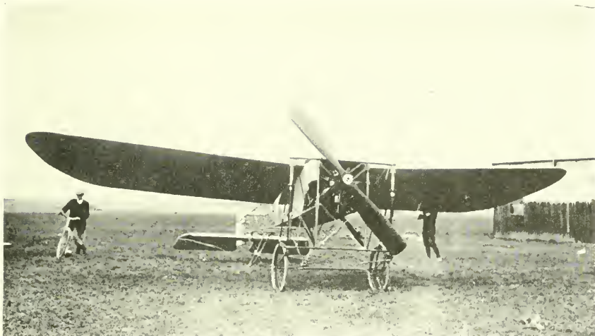
1. The 1909 Bleriot monoplane. Tractor engine location, warping wings for lateral control, rear elevators and tail.
