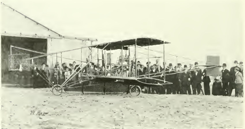
2. The 1909 Curtiss biplane. Engine back of pilot, interplane ailerons, shoulder yoke controls, three-wheel and skid landing gear, and rear elevators.
