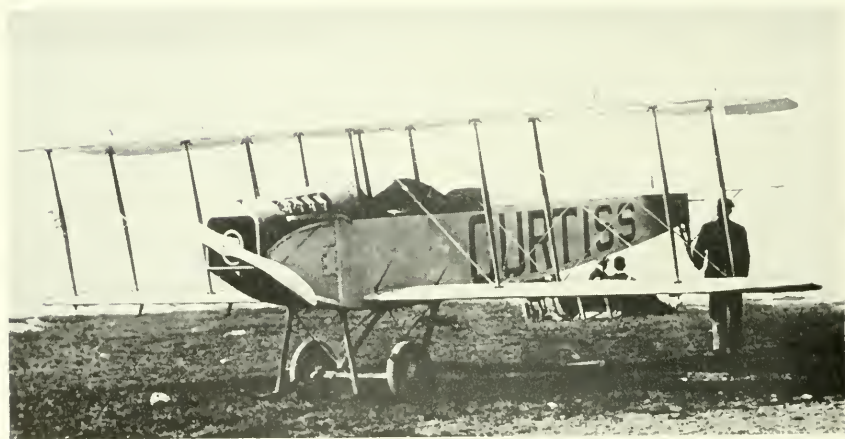
2. This 1913 Curtiss tractor had a typical landing gear of skids and wheels. On a hard landing, the skids would break and turn the plane over.
