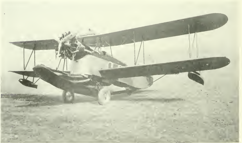
2. The practical retractable gear of the amphibian in 1923-1933 led to a much wider adoption of this feature on land planes.
