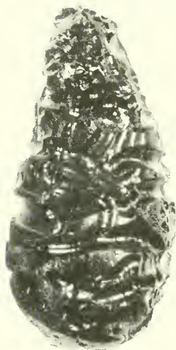
2. Billitonites from the island of Billiton, illustrating the wormlike grooves and navels resulting principally from chemical corrosion through being buried in moist soil for many years.
