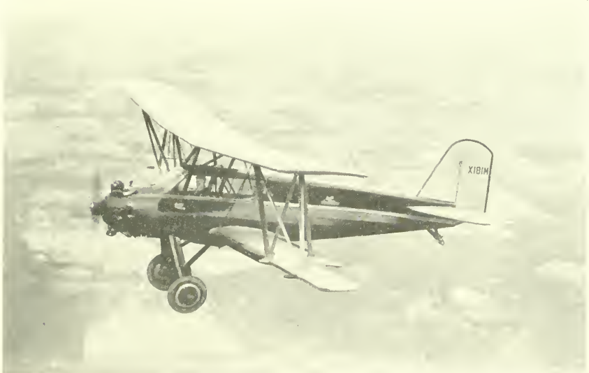
2. The Curtiss Tanager, winner of the Guggenheim Safe-Aircraft Competition of 1929. Outboard ailerons on lower wings, complete slots and flaps. This plane had by far the best speed range up to that time.
