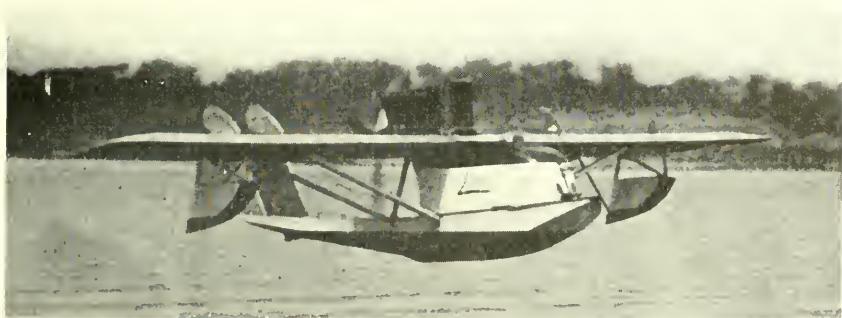
2. The Loening Air Yacht of 1921, Collier Trophy winner. The monoplane structure was strong, simple, and efficient, but not popular enough for acceptance at the time.
