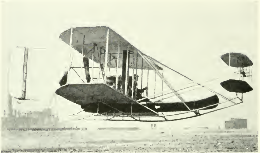
1. The Wright Model A of 1909, with canoe attached for Hudson-Fulton flights over New York harbor. Skid landing gear, no wheels, no rear horizontal tail.
