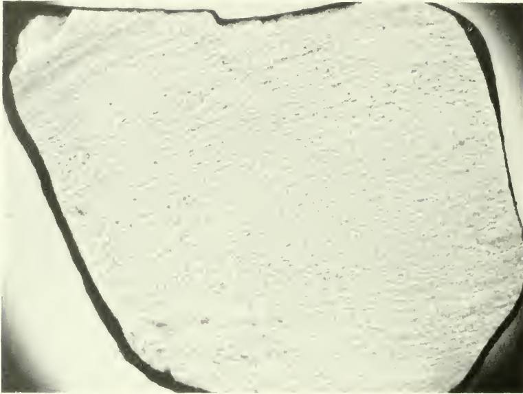
2. Libyan Desert glass, showing internal structure of a thin polished section by means of transmitted light.
