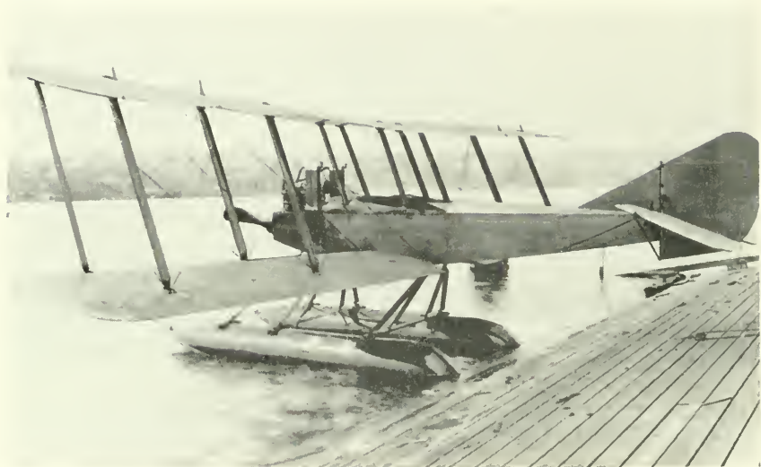
1. An early Boeing training plane. Note low rudder, small fin, short tail length, no stabilizer. This was typical of the 1910-1914 era.
