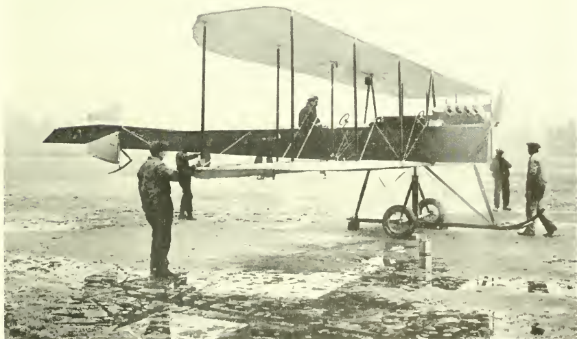
2. An early French innovation that marked the start of an era, the Astra tractor of 1911, with Wright biplane wings on a covered fuselage, and Renault tractor engine and propeller.
