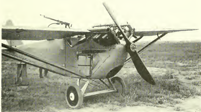
1. The Loening monoplane of 1918. The first rigid strut-braced wing structure, not widely used until 20 years later.
