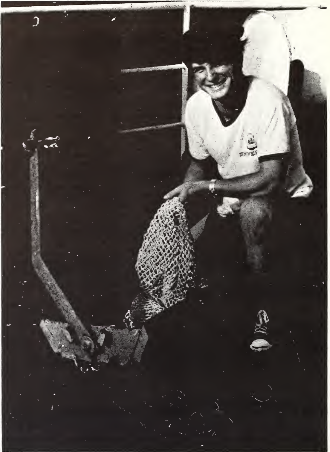
Figure 9. A dredge which is dragged along the bottom on a cable from a ship to recover loose rocks.
