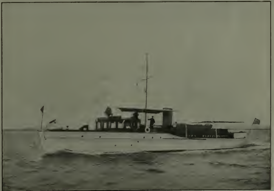
Large gasoline cruiser which is qualified to hold the sea under all ordinary conditions. She has an 84-foot waterline
