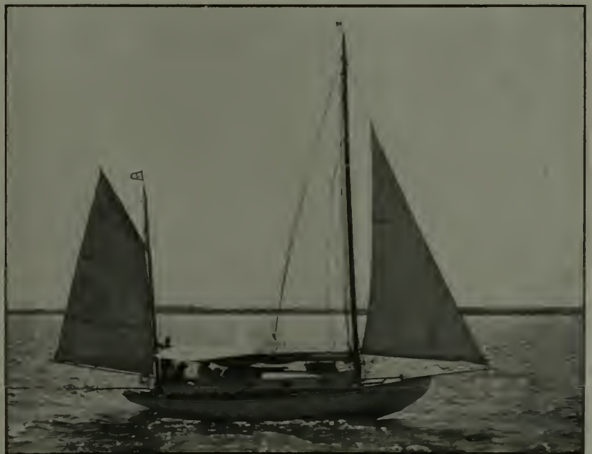
A popular type of cruiser is the auxiliary yawl which can defy the doldrums and go to port under power
