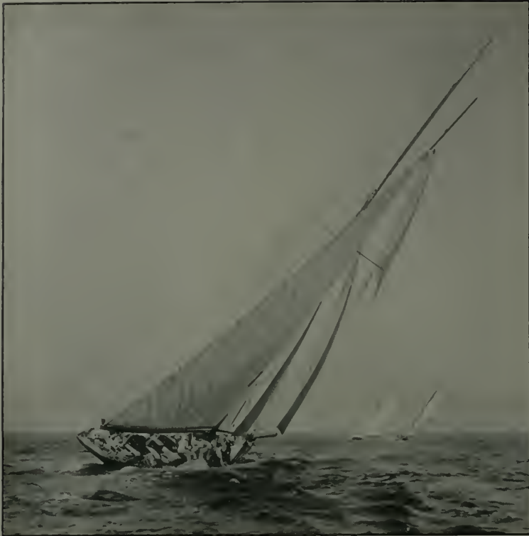
Close hauled. A large racing sloop with lee scuppers awash. She is sailing to windward
