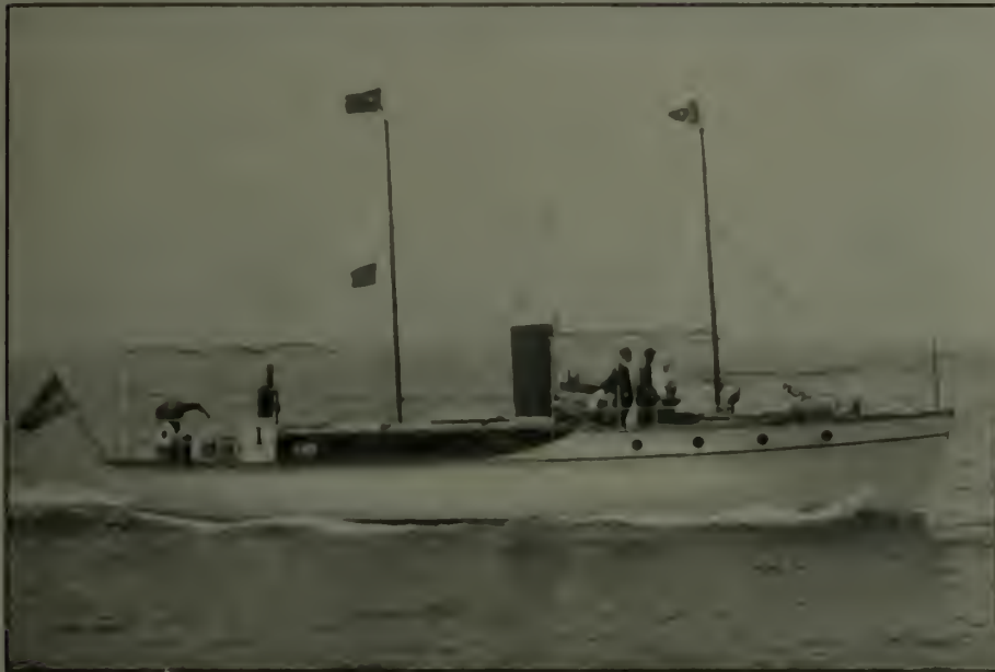
High deck off-shore motor boat, which has been designed and built to cruise or race over coastwise routes
