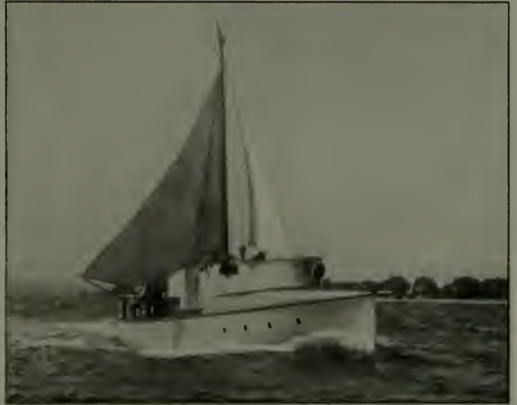
Ocean going motor racer starting on Bermuda race. Note auxiliary sails and bridge protection
