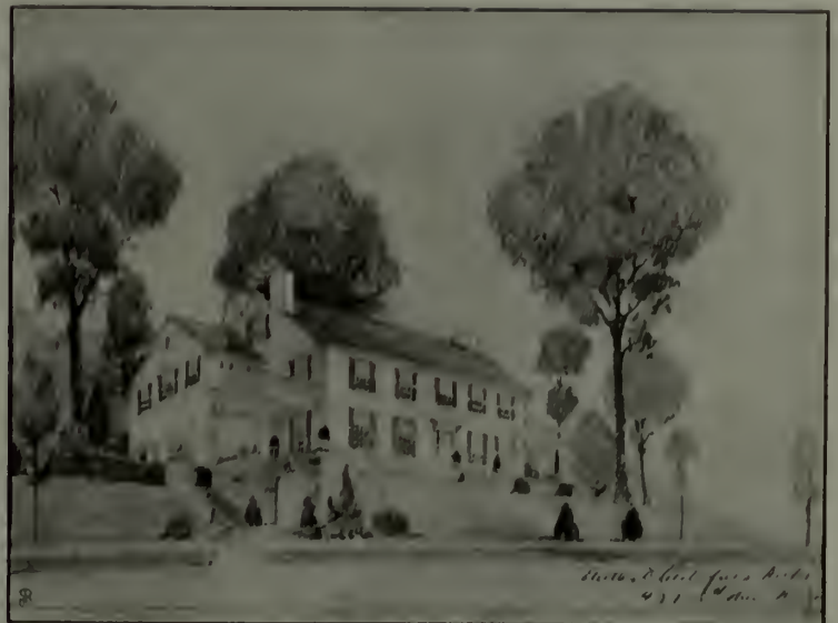
House at Kew, Long Island, designed by Electus D. Litchfield. Different levels in the lot allow of picturesque terracing and making the garage a part of the terrace and basement
