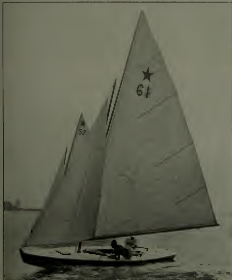
The Star class of sloops is extremely popular on Long Island Sound, where clouds of them race every summer. It will be noted that while of scow or "sidewalk" construction, they have pointed bows—this for rough weather.
