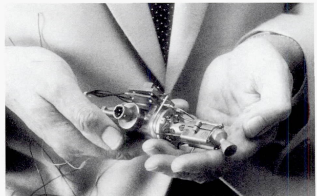
THRUSTER ENGINES, like this one-pound model, are used to keep TDRSS satellites from drifting from the precise positions they must retain for their work. This
