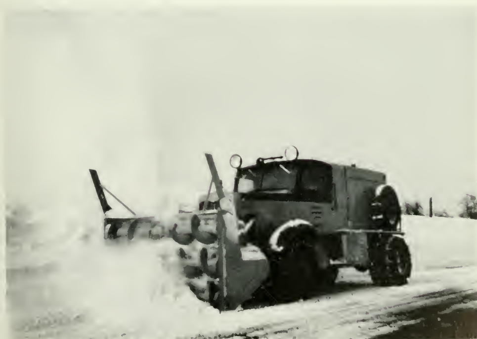
Close-up view of rotary plow in operation.
