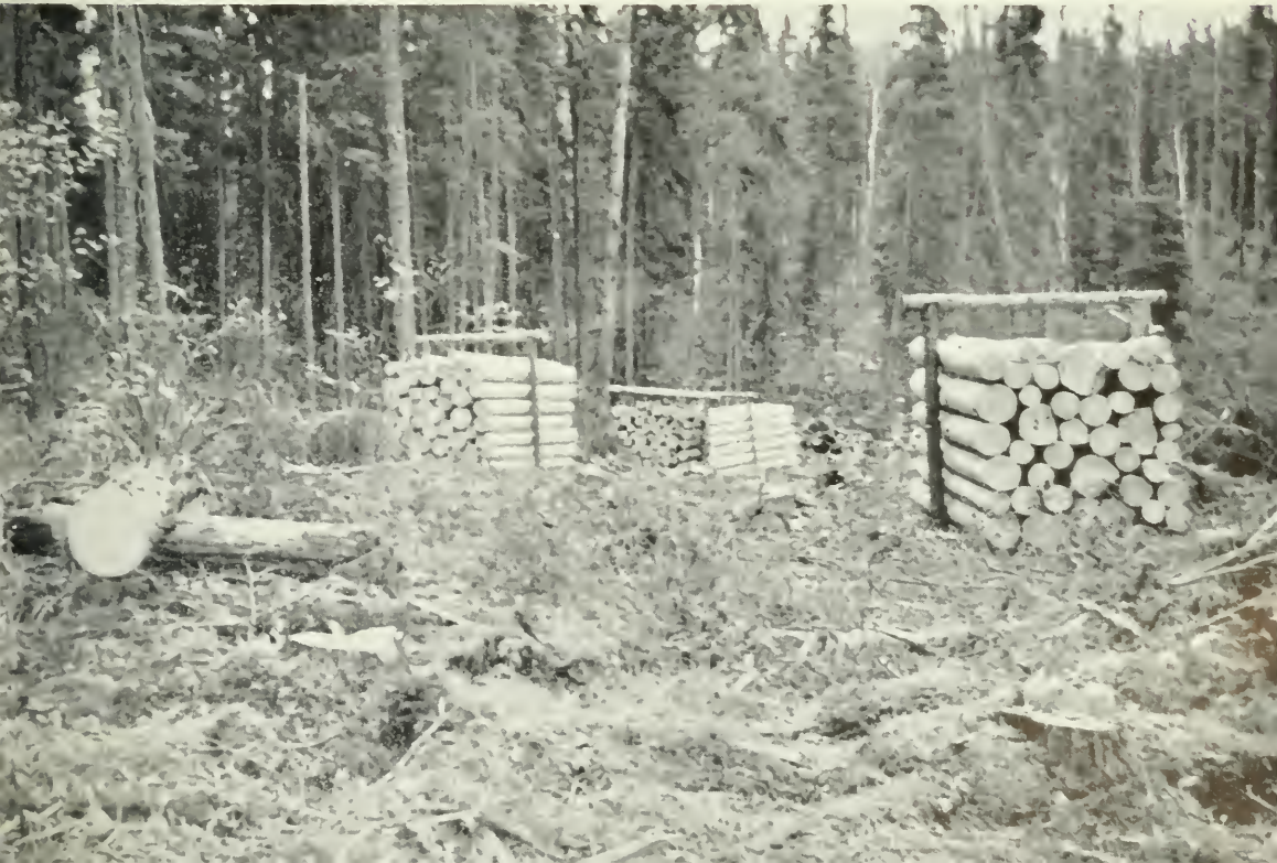
Nine-inch dry spruce top wasted because it was difficult to peel. (Pulpwood-exporting company operation.)
