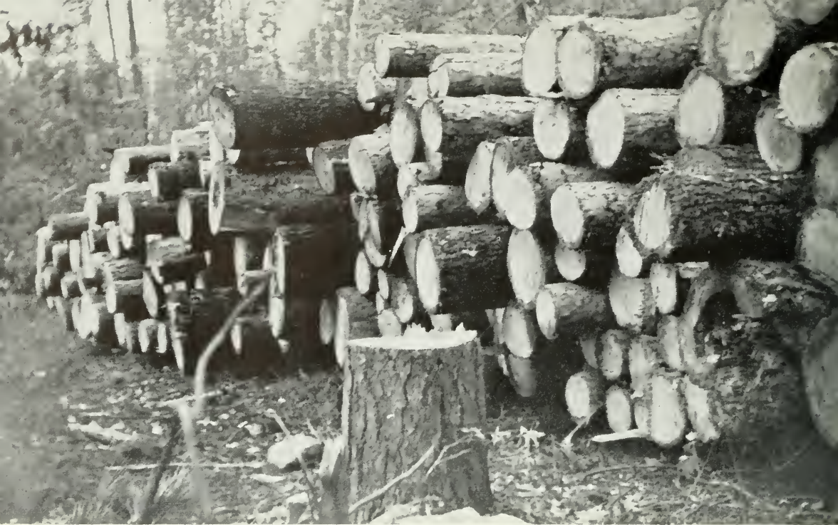
A poorly built skidway of pine sawlogs. Ends are uneven, thus making proper measurement of either diameters or lengths impossible.
