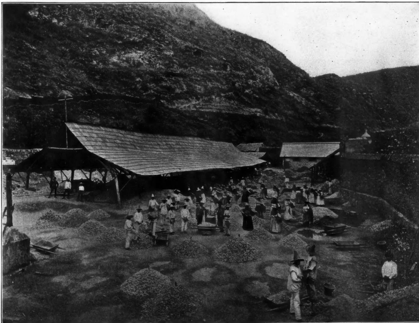
ORE YARD AT THE SIRENA MINE, SHOWING THE MEN AND WOMEN SORTERS.
