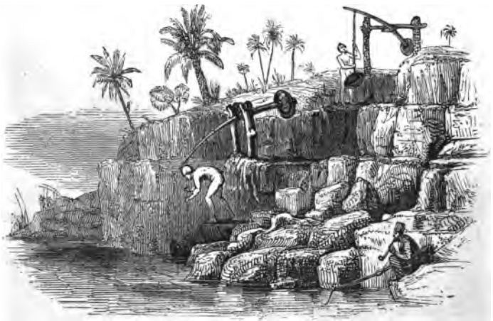
a. Modern shadoof , or pole and bucket, used for raising water, in Upper and Lower Egypt.
