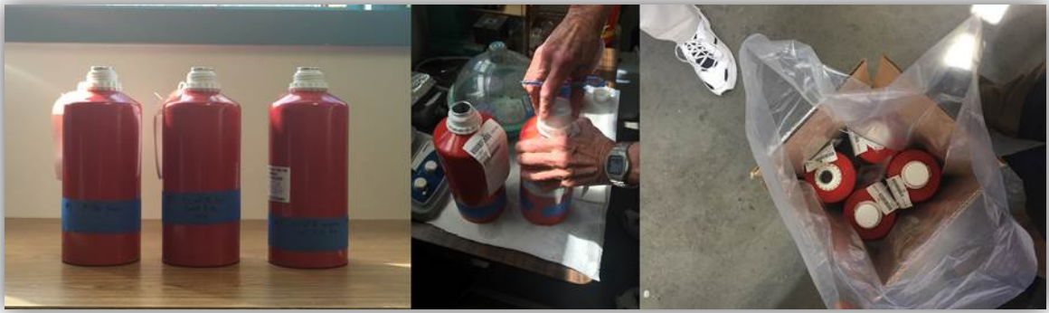
Figure 15. Containers Used to Transport F-76, 0.1wt% GO/F-76 Mixture, and 0.1wt% G/F-76 Mixture
