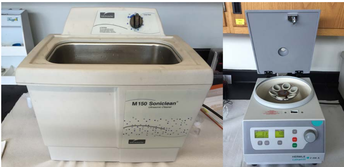
Figure 5. MIDMARK M150 Soniclean Ultrasonic Cleaner (Left) and HERMLE Labnet Z206A Centrifuge (Right)
