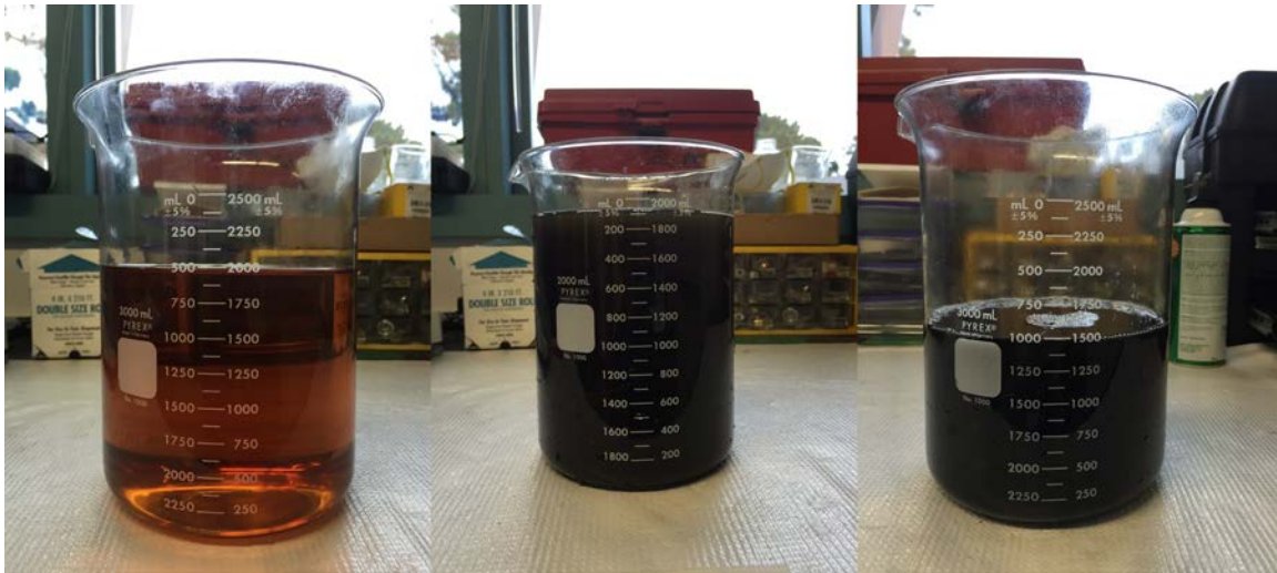
Figure 38. (Left to Right) 2000 ml F-76, 2000 ml 0.1wt% GO/F-76 Mixture, and 1500 ml 0.1wt% G/F-76 Mixture
