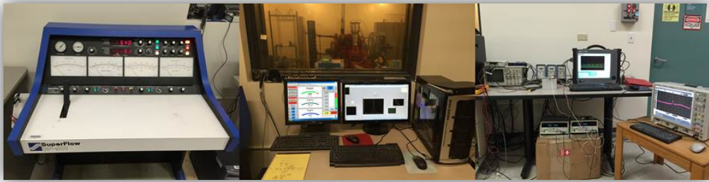
Figure 17. Diesel Engine Test Stations (Left to Right): Engine Speed/Load Console, Engine Speed/Load Analyzer, Engine Cylinder Analyzer
