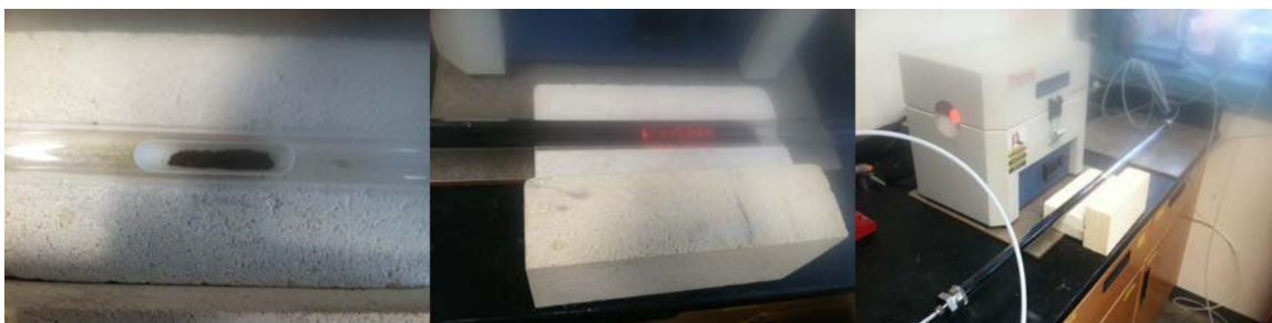
Figure 7. (Left to Right) GO in Quartz Tube Prior to Thermal Exfoliation, Graphene just after Thermal Exfoliation, ThermoScientific Furnace with Graphene in Quartz Tube
