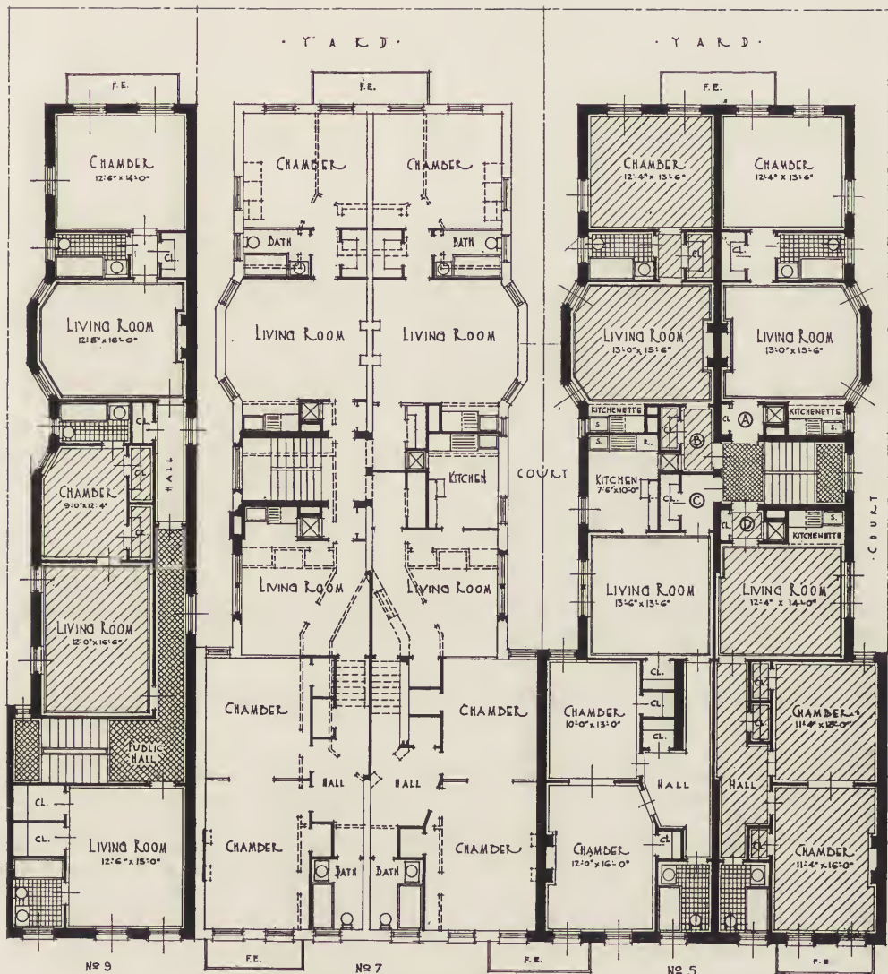
PLAN SHOWING ALTERATIONS IN BUILDINGS NO. 5 & NO. 7
