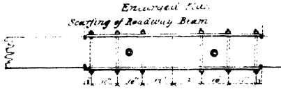
Enlarged Elevation Scarfig of Roadway Beam.
