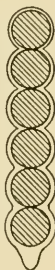
FIG. 33. — Diagram showing the adjustment of the capillary film in a long column and the appearance of free or gravitational water if the weight is too great for the supporting films.
