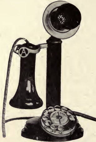
FIG. 43.—AUTOMATIC TELEPHONE STATION
