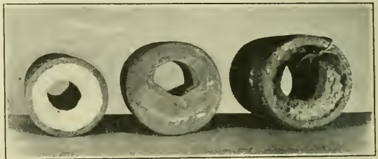
SCALED NIPPLES THE ONE ON THE RIGHT SHOWS THE RESULT OF ONE MONTH'S RUN.
