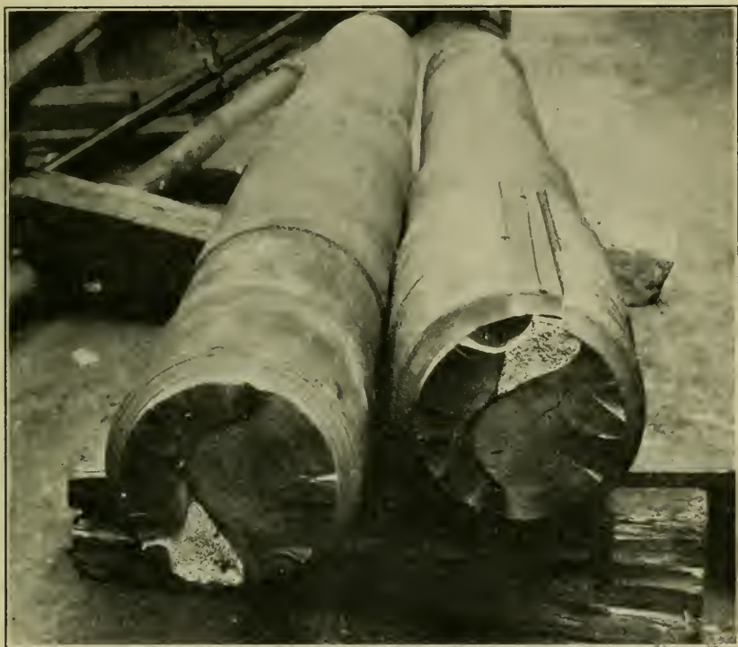
FAILURE OF SHAFT CAUSED BY WELDING.
