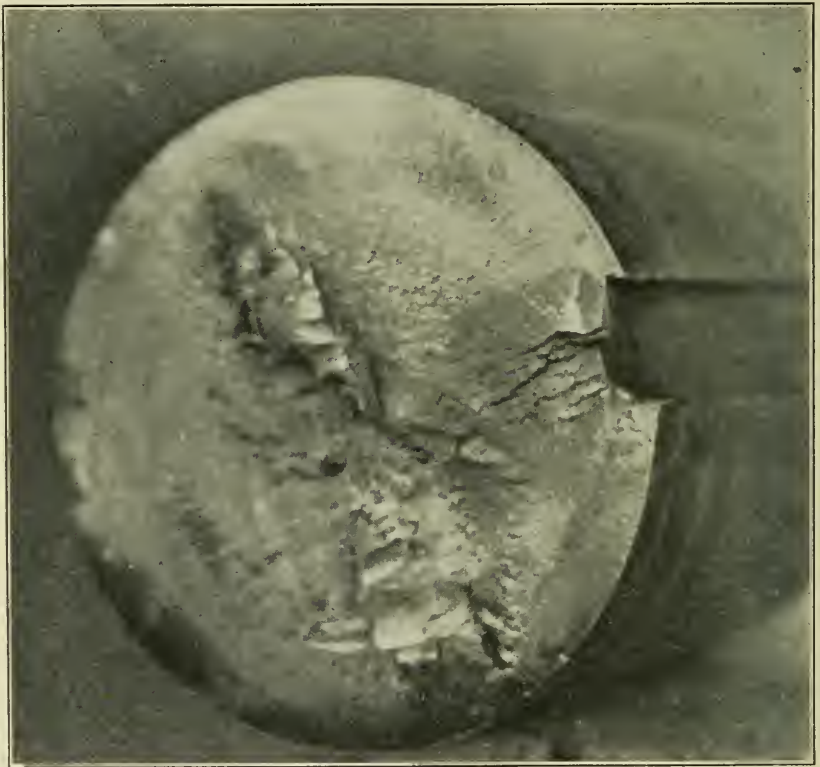
FRACTURE OF ENGINE SHAFT.
