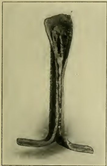
A CORRODED STAY.
