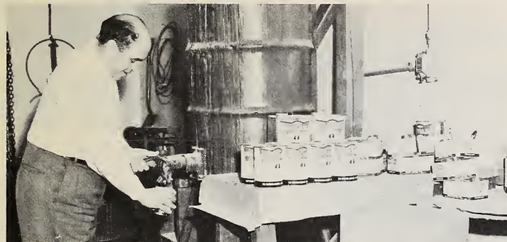
The contact cement is removed directly from the mixing machine into tin containers.
