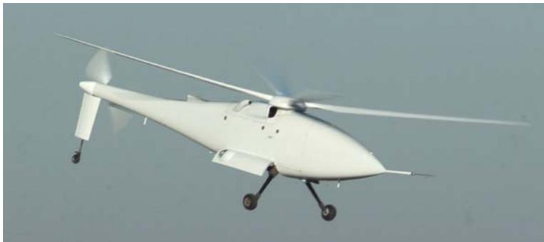
Figure 24: A-160 vertical take-off and landing (VTOL) unmanned air vehicle (UAV).
