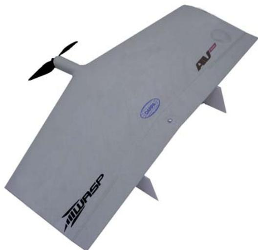
Figure 20: Wasp micro air vehicle.
