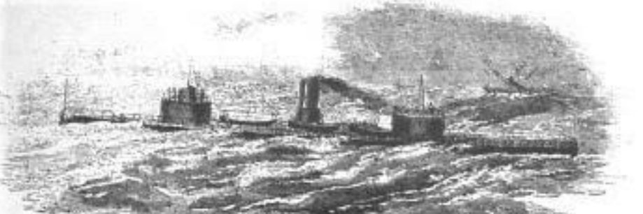
THE "ONONDAGA" Iron-clad Battery, 4 guns, 1250 tons, length 225 feet, breadth 50 feet. Built by T. F. Rowland, Greenpoint, L. I. Launched July 17, 1863.
