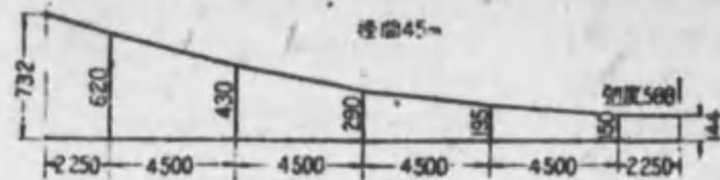
吊架線張力 架空電車線 170 mm 2 渡付硬鋼線の場合 1000 kg 15°C 無水無風 110 mm 2 " " " " " " 775 kg " " " " " " " " " " " "
