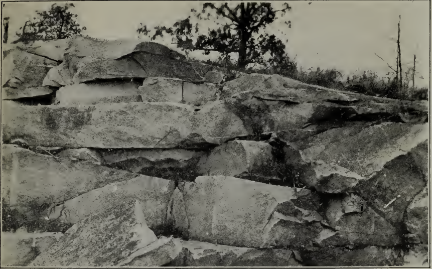
A. GRANITE OUTCROP AT MEYERS QUARRY NEAR PIERZ, MORRISON COUNTY, SHOWING HORIZONTAL JOINTING PHOTO BY CARL ZAPPE
