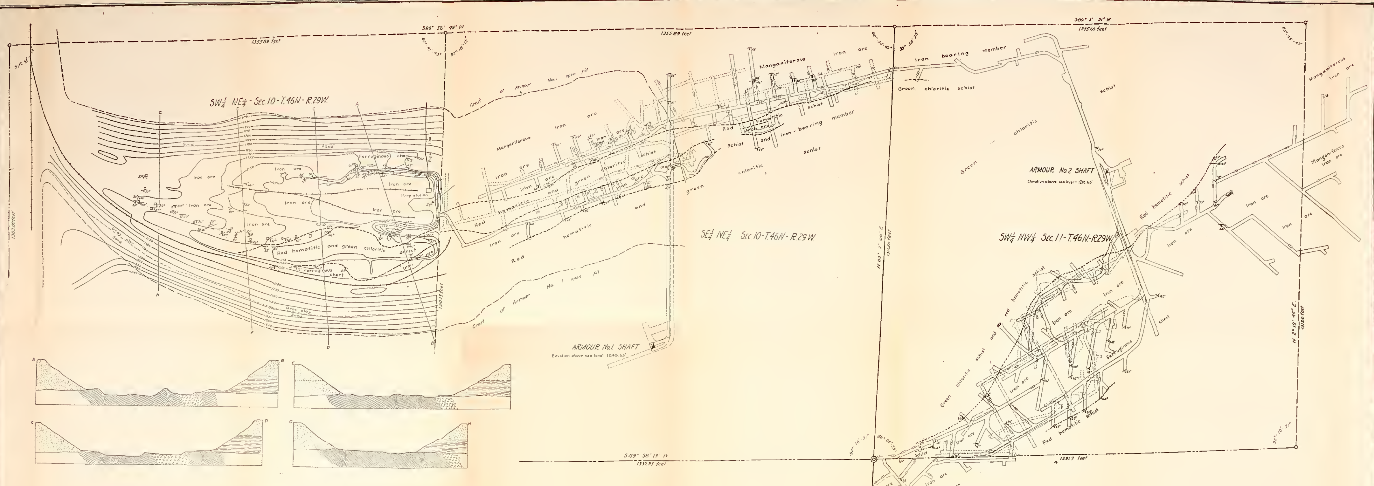
MAP AND SECTIONS SHOWING THE GEOLOGY AND WORKINGS OF THE PENNINGTON, ARMOUR No. 1, AND ARMOUR No. 2 MINES CUYUNA IRON-ORE DISTRICT MINNESOTA Surveyed in July, 1915
