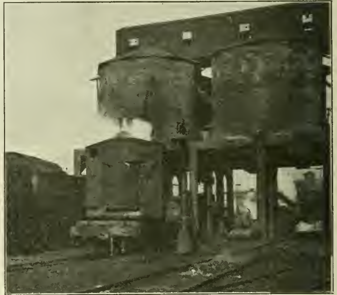
Modern Arrangement by which Locomotives Can Take Water and Coal at the Same Time
