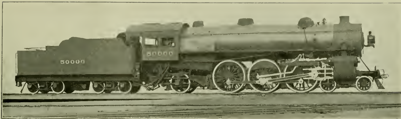
Experimental Pacific Type No. 50000, Which Established New Records for Power per Unit of Weight
