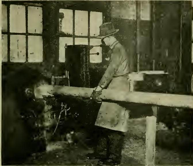
Fig. 8—Machines for Safe Ending Superheater Flues Are Located So That the Operator Has to Move the Tube Only a Slight Distance to Complete All the Operations
