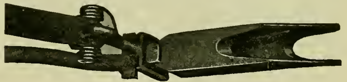
Fig. 3—Device for Distributing Oil to the Flange
