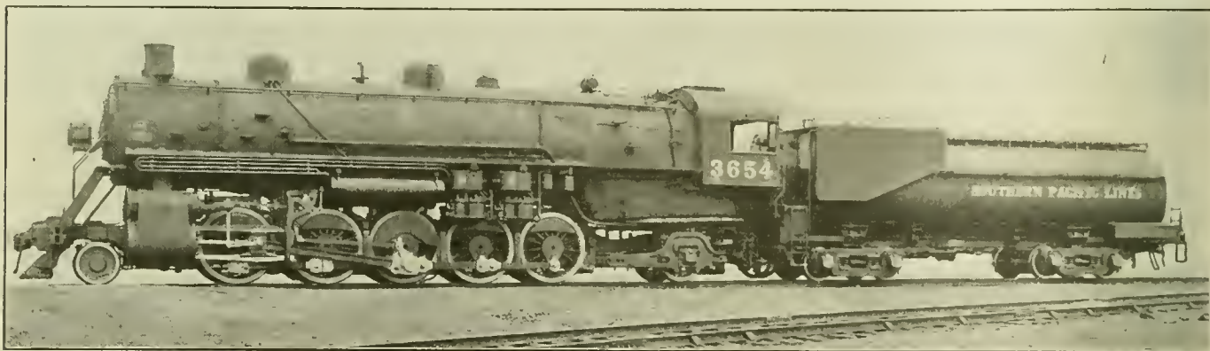
2-10-2 Type Locomotive for Handling 1,000 Tons on 2.4 Per Cent Grades
