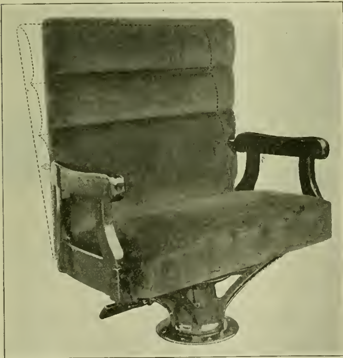
Fig. 1—Normal and Inclined Positions of Smolar Car Seat
