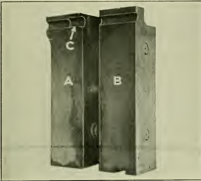
Fig. 7—Extension Dies for Forming Second Upsetting Operation on Brake Shafts
