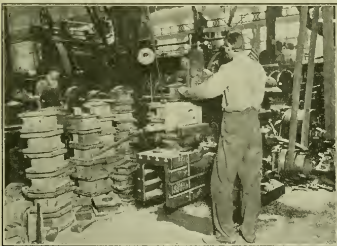
Main Rod Brasses, Machined in Shop Order Lots of 30 Pairs
