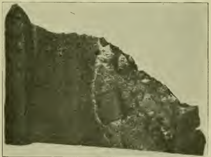
Fig. 14—Example of Metal Too Poor to Weld
