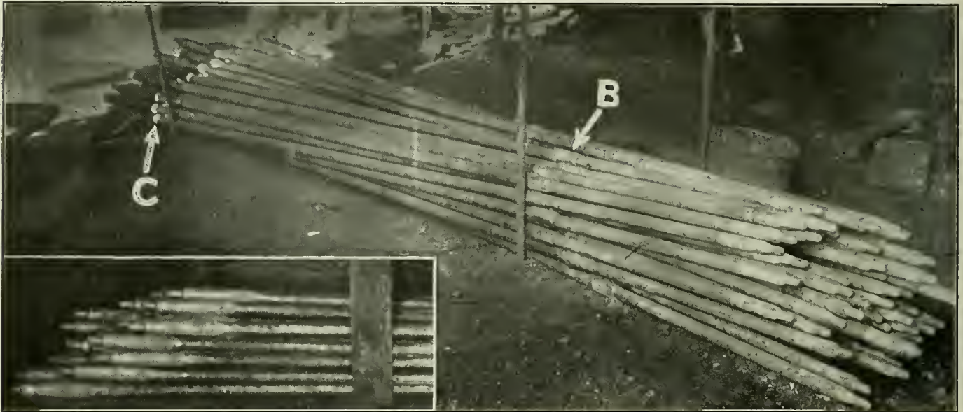
Fig. 4—Finished Brake Shafts Upset at Two Points, 5 Ft. 7\frac{1}{4} In. Apart
