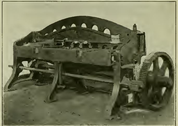
Heavy Shear Repaired by Welding
