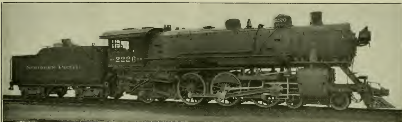
Heavy Pacific Type Handles 12 Passenger Cars or More Over the Rocky Mountains
