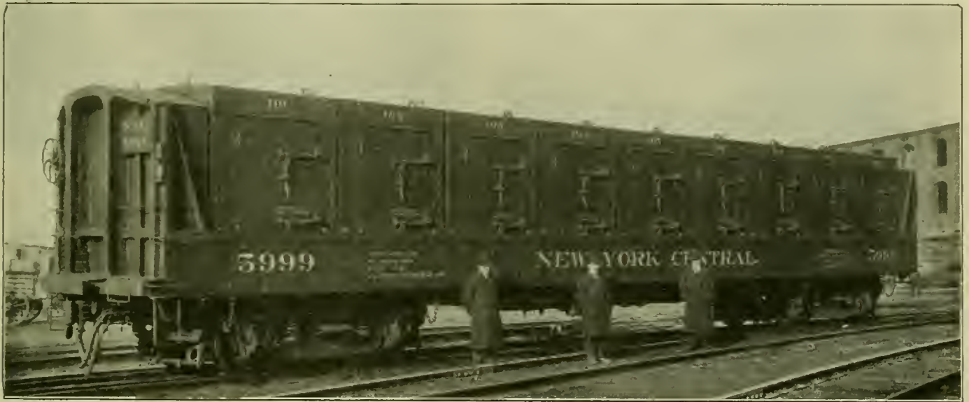
New York Central Container Car Designed for Handling Express Matter, Equipped with Passenger Trucks and Buffers and with Air, Steam and Signal Line for Passenger Train Operation
