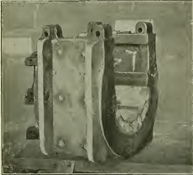
Driving Box Shoe and Wedge Liner Tack-Welded in Place
