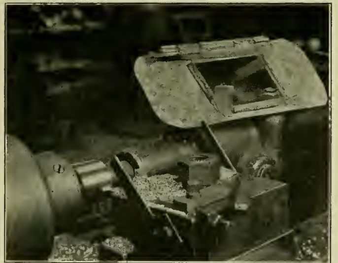
Fig. 3—Method of Machining Washout Plugs
