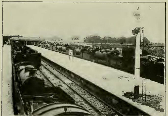
Idle Locomotives—Built in England for War Service in France—Too Heavy for Service in England
