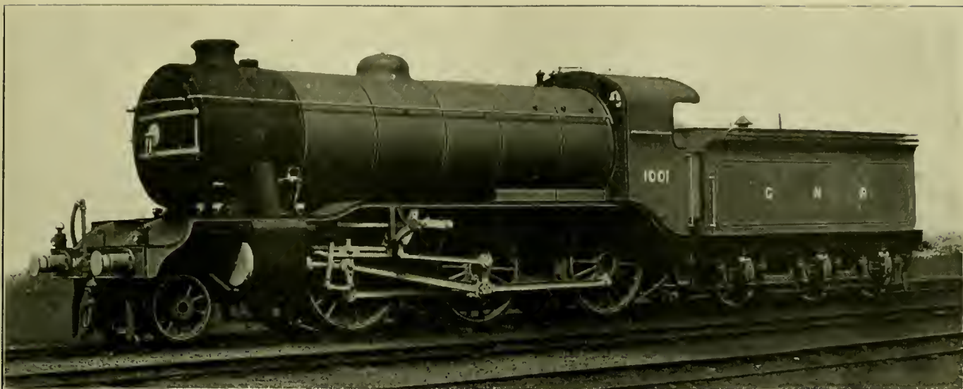
Great Northern Railway Three-Cylinder Type Locomotive for Fast Freight Service, Designed by H. N. Gresley, Locomotive Engineer, Built 1920, Doncaster Shops
