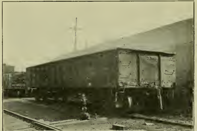
Fig. 3—Car Shown in Fig. 2 After Being Straightened
