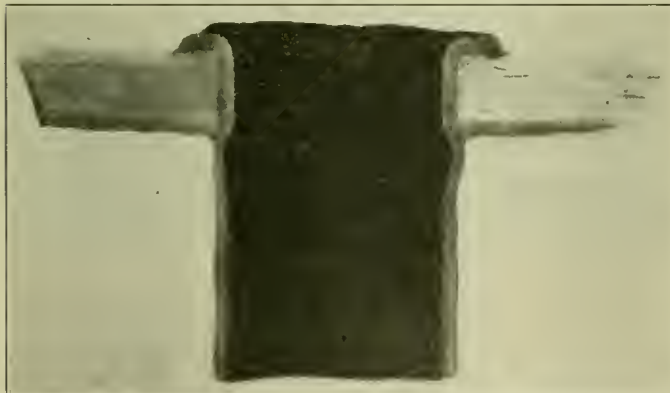
Fig. 13—Etched Section Through a Boiler Tube Welded to the Sheet; Metal of the Sheet Unaffected
