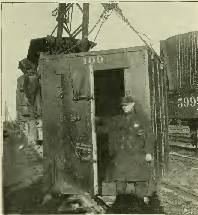
Empty Container Showing Interior and Door Construction
