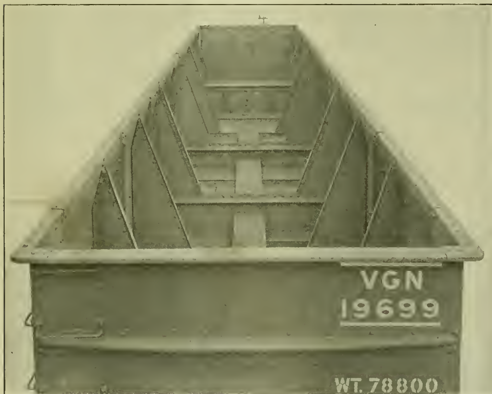
Interior of the Car Body. Showing Gusset Side Stakes, Bolsters and Cross Bearers
