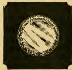
FIG. 4.—Plan of the bottom of safety-valve, the bright portion being indicated by the white arc. "It did not leak." (P)
