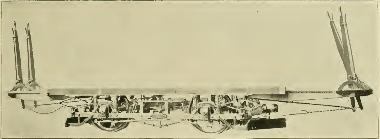
SHOWING ARRANGEMENT OF LEVER BRAKES ON WILMINGTON CITY RAILWAY.
