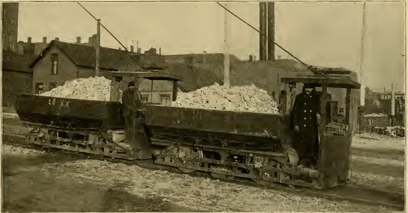
TROLLEY ORE CARS—BUTTE CONSOLIDATED RAILWAY COMPANY, BUTTE, MONT.
