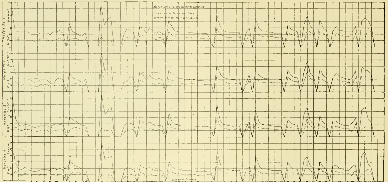
THE TWO ABOVE CURVES ARE FROM THE SAME RUN—MADE TO DETERMINE THE VOLTAGE AND CURRENT DISTRIBUTION BETWEEN THE FOUR MOTORS OF AN EQUIPMENT.
