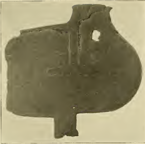
FIGURE 2—SECTION OF OLD "CAST-WELD" JOINT SHOWING CLEARANCE BETWEEN IRON AND RAIL.
