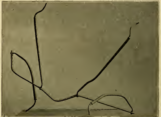
DASH RAIL BENT BY CYCLONE.
