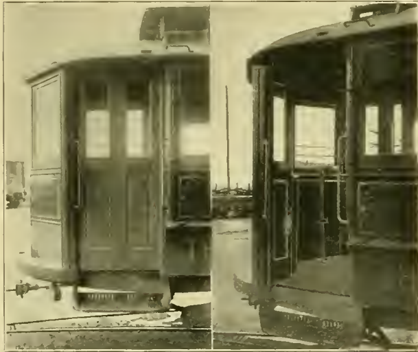
CALUMET VESTIBULE ON NEW CARS—FOLDING DOOR SWINGS FORWARD.
